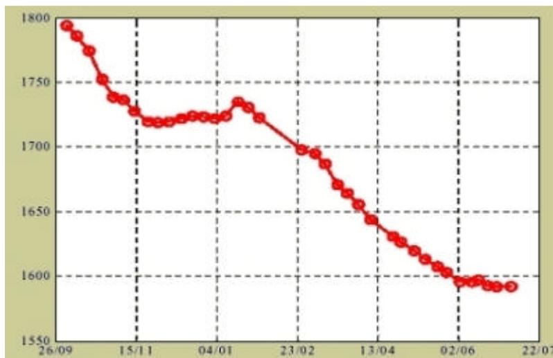
Degradation in Power Output from Solar Panels since Launch
