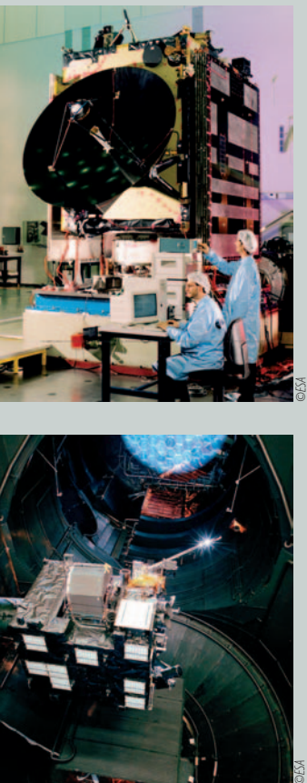
The Rosetta spacecraft without thermal blankets ready for vibration testing on the shaker (top), and with thermal blankets ready for testing in the Large Space Simulator (bottom), at ESTEC in The Netherlands
