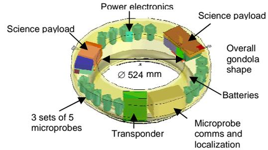
Figure 4: VEP aerobot gondola
