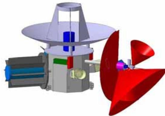
Figure 12: IHP Science configuration with payload field of views
