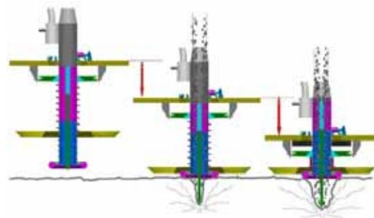
Figure 7: DSR pneumatic sampling mechanism
