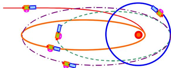
Figure 5: DSR Mars insertion and co-orbit with Deimos
