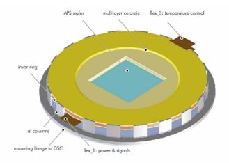
Figure 5.1.1 – Reference design of the WFI Focal Plane Assembly.
