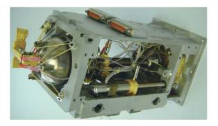
Figure 4.2.2 – Herschel sorption cooler potentially re-usable onboard XRO (courtesy of *CEA-CBT*).
