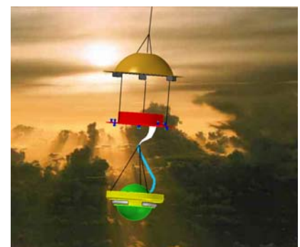
f.) Inner structure release and start of balloon deployment.
