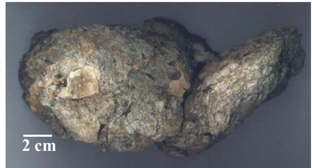
Fig. 2. Thermally altered cobbles, indented into each other and cemented by silicate melt
