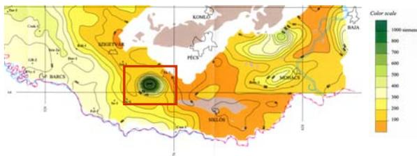
Fig. 1. The telluric conductivity anomaly at Magyarmecke, Hungary, on the Telluric Conductance Map of Transdanubia ([2])
