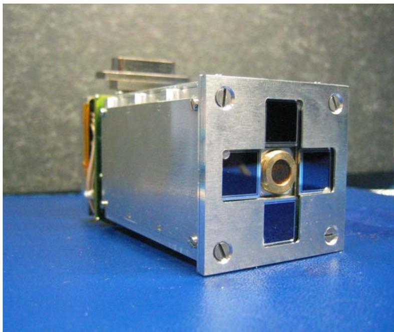
Figure 6 MIMOS sensorhead (detectors visible)
