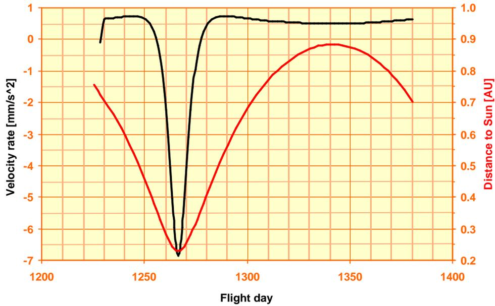
Figure 2-10. Ballistic transfer, 2013 launch: velocity rate toward the Sun [ $\text{mm/s}^2$ ] and distance to Sun centre during first revolution after Venus GAM 2.
