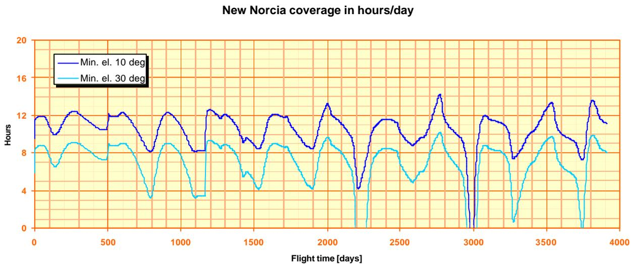
Figure 2-21. Ballistic transfer, 2015 launch: coverage in hours/day from New Norcia function of flight day.
