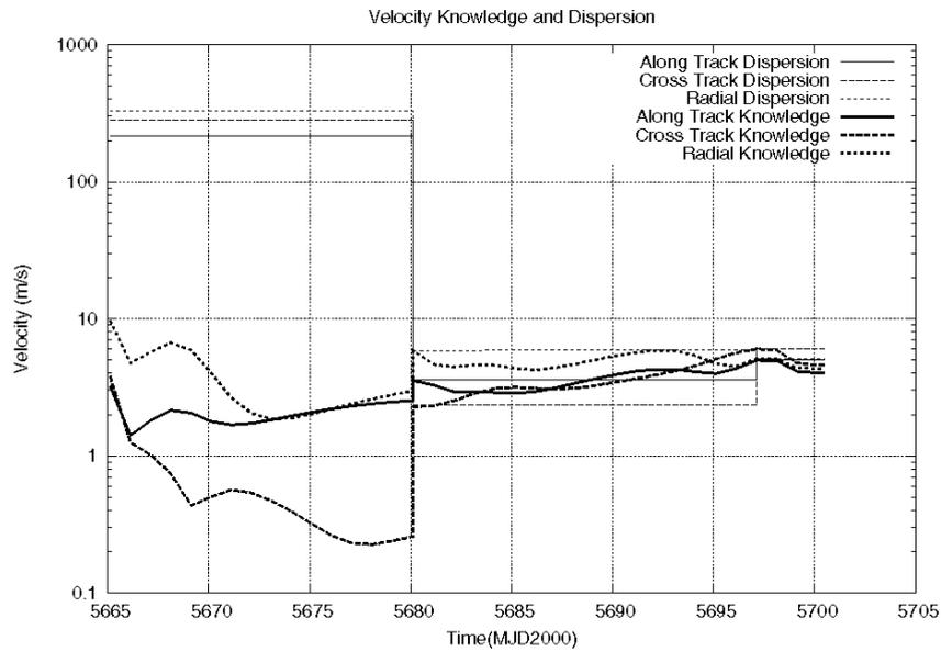
Figure 4-2. Evolution of the  $1\sigma$  velocity knowledge (thick lines) and dispersion (thin lines) mapped to the pericentre (GAM V2).
