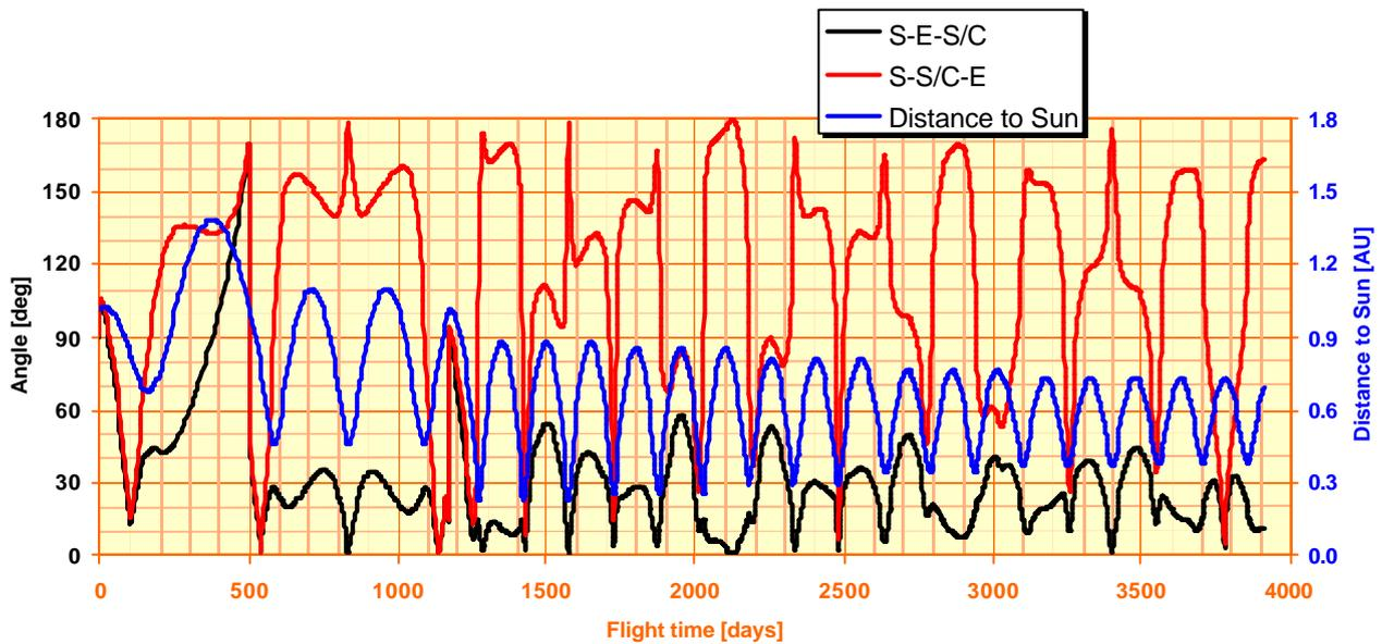
Figure 2-17. Ballistic transfer, 2015 launch: angle Sun-Spacecraft-Earth and Sun-Earth-Spacecraft and distance to Sun centre [AU] function of flight day.
