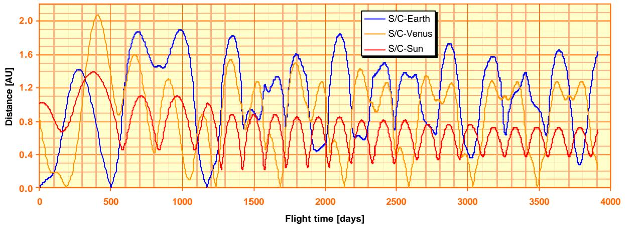
Figure 2-16. Ballistic transfer, 2015 launch: distance of the spacecraft from Earth, Venus and Sun function of flight day.
