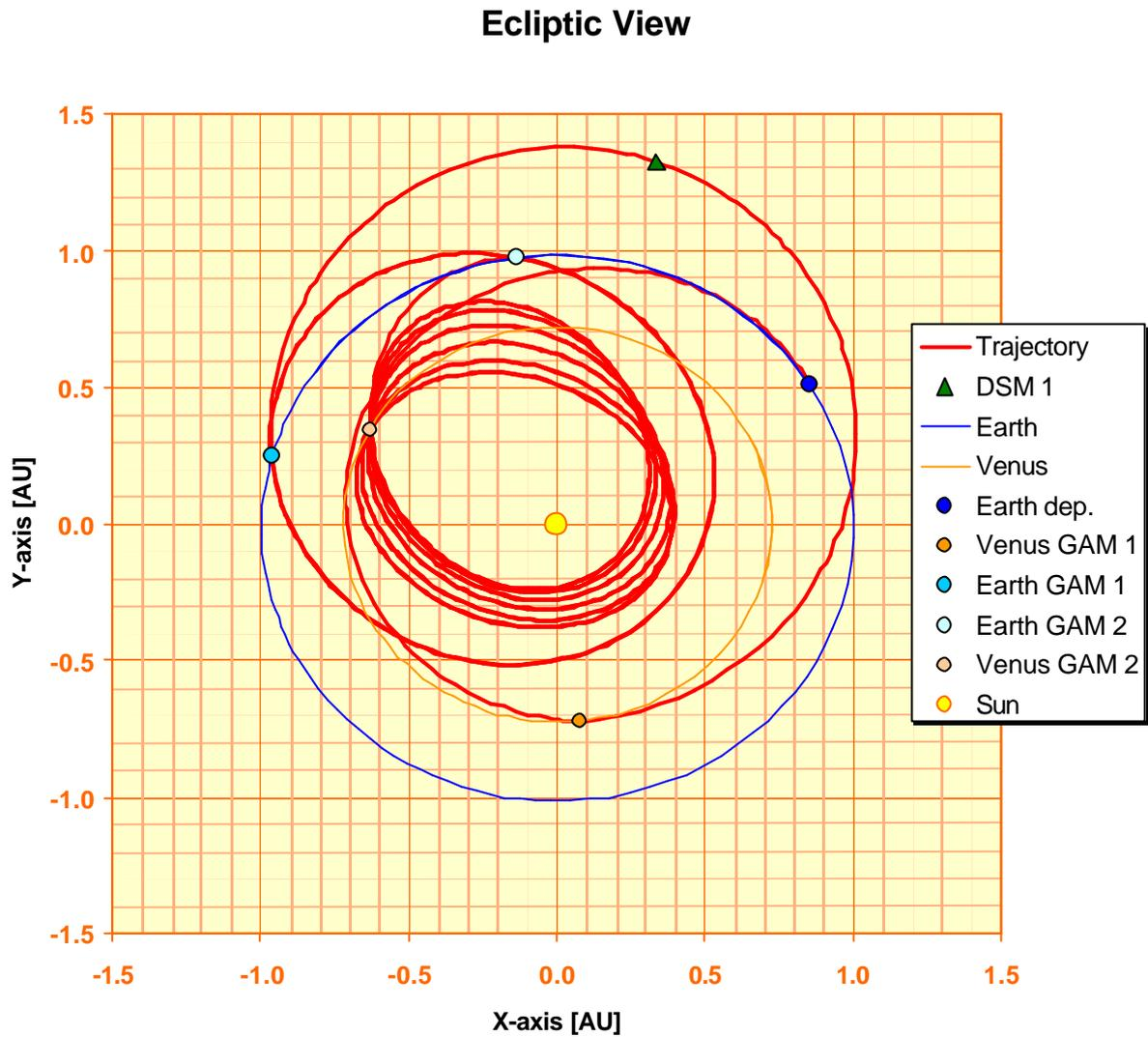
Figure 2-1. Ballistic transfer, 2013 launch: ecliptic view of the trajectory, GAMs until Venus GAM 2 and DSM.
