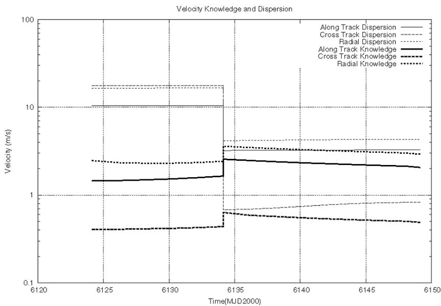
Figure 4-5. Evolution of the  $1\sigma$  velocity knowledge (thick lines) and dispersion (thin lines) mapped to the pericentre (GAM V3).
