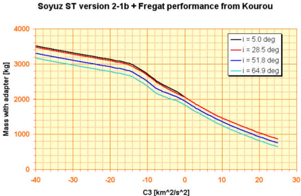
Figure 5-1. Soyuz/ST + Fregat performance (kg, including adapter) for highly elliptic (perigee height 200 km) and escape missions in terms of  $C_3$  for a launch from Kourou with inclination  $i = 5^\circ$ ,  $28.5^\circ$ ,  $51.8^\circ$  and  $64.9^\circ$  (Ref. 3).
