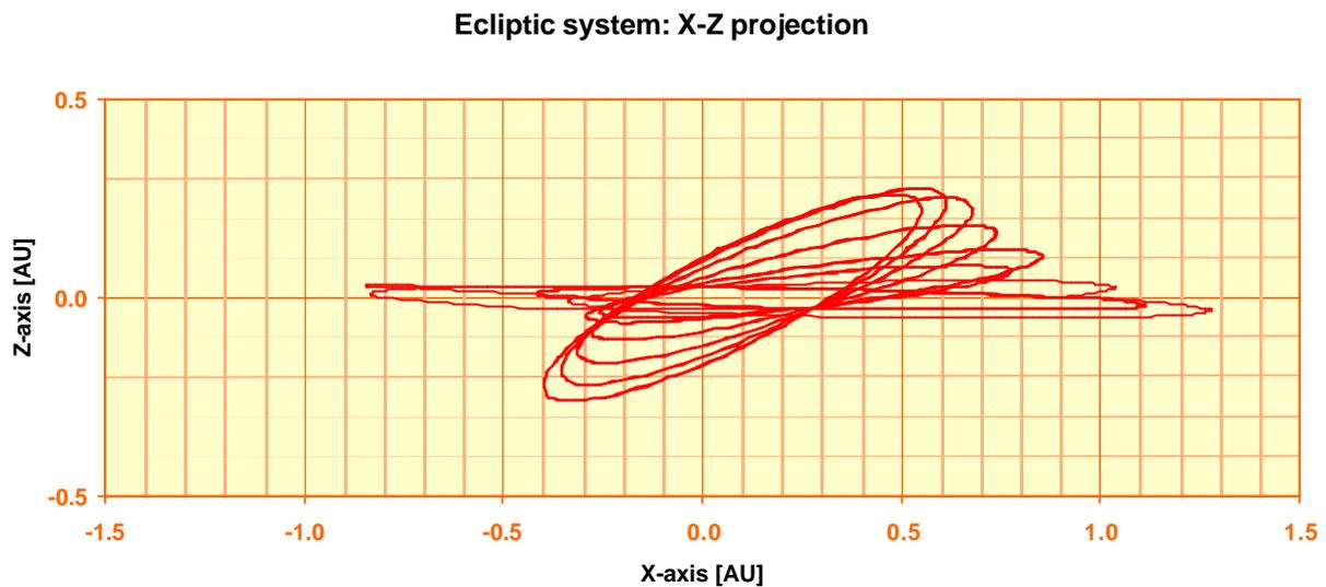
Figure 2-25. Ballistic transfer, 2017 launch: projection of the trajectory on the ecliptic system (x, z)-plane.
