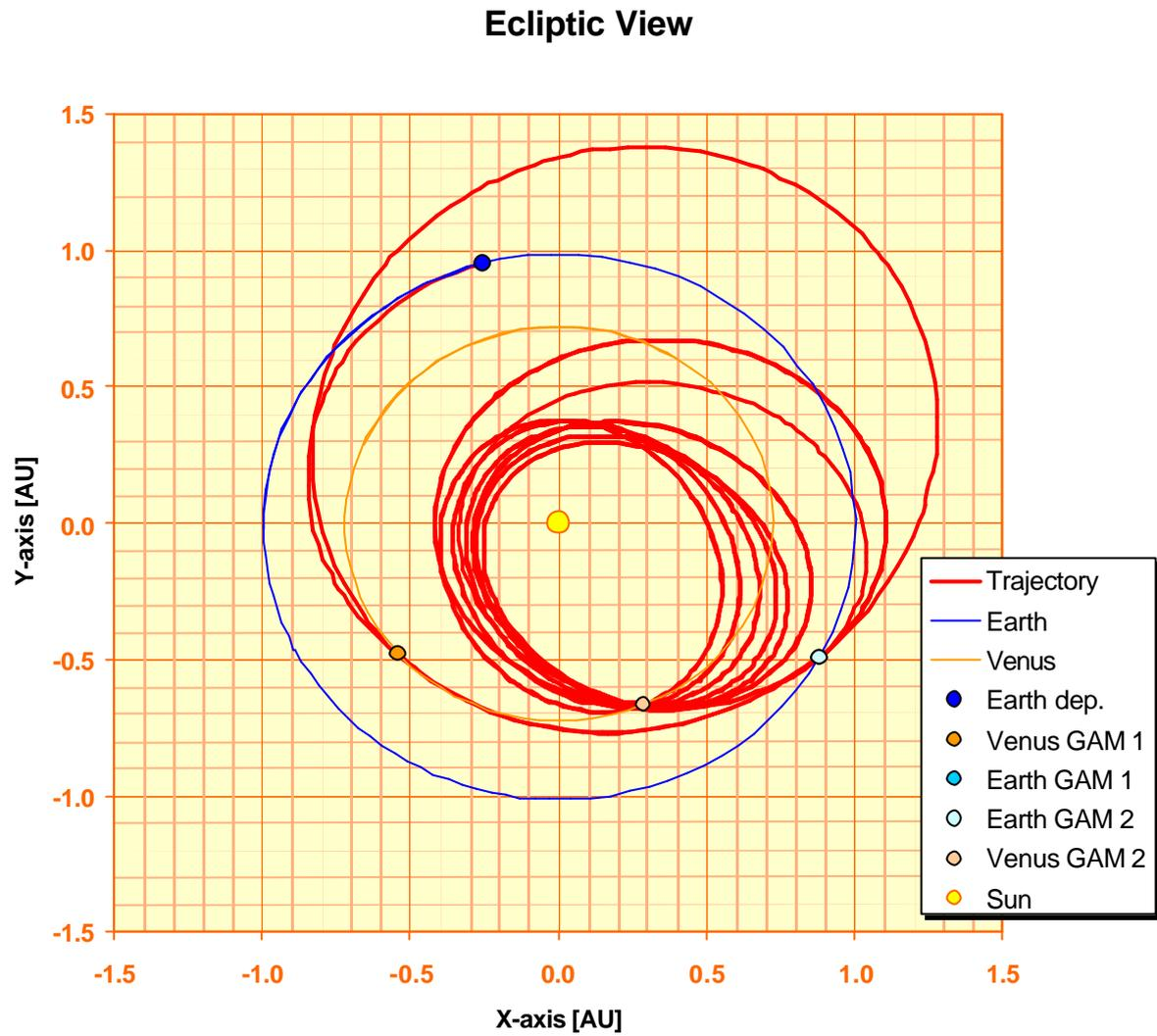
Figure 2-23. Ballistic transfer, 2017 launch: ecliptic view of the trajectory, GAMs until Venus GAM 2 and DSMs.
