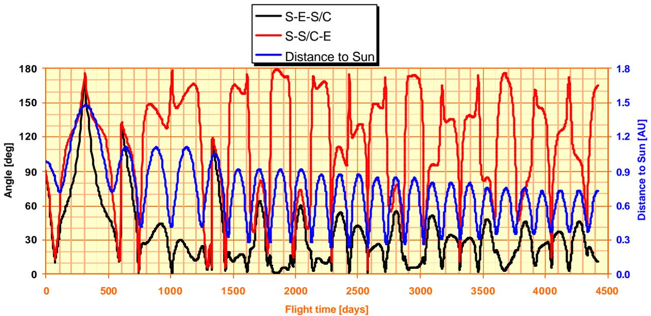
Figure 2-27. Ballistic transfer, 2017 launch: angle Sun-Spacecraft-Earth and Sun-Earth-Spacecraft and distance to Sun centre [AU] function of flight day.
