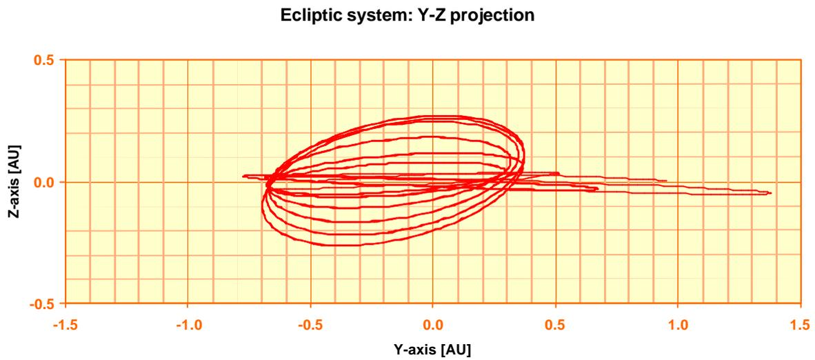
Figure 2-24. Ballistic transfer, 2017 launch: projection of the trajectory on the ecliptic system (y, z)-plane.
