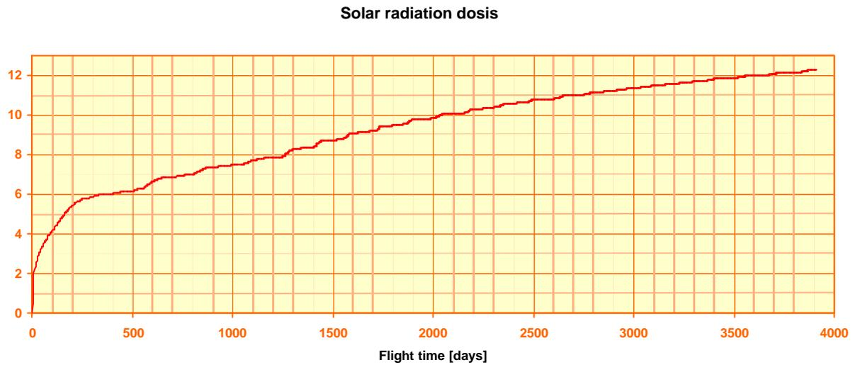
Figure 2-20. Ballistic transfer, 2015 launch: solar radiation integrated doses function of flight day.
