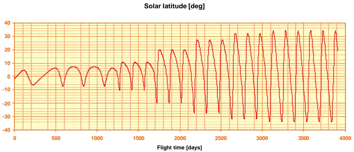
Figure 2-18. Ballistic transfer, 2015 launch: solar latitude function of flight day.
