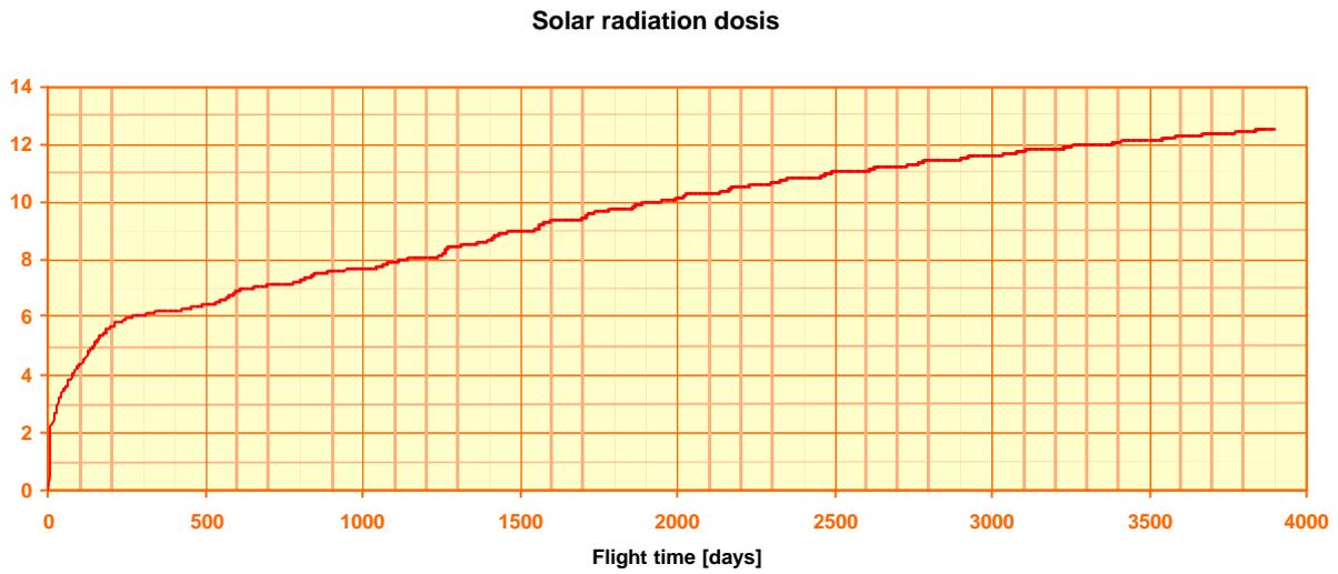
Figure 2-8. Ballistic transfer, 2013 launch: solar radiation integrated doses function of flight day.
