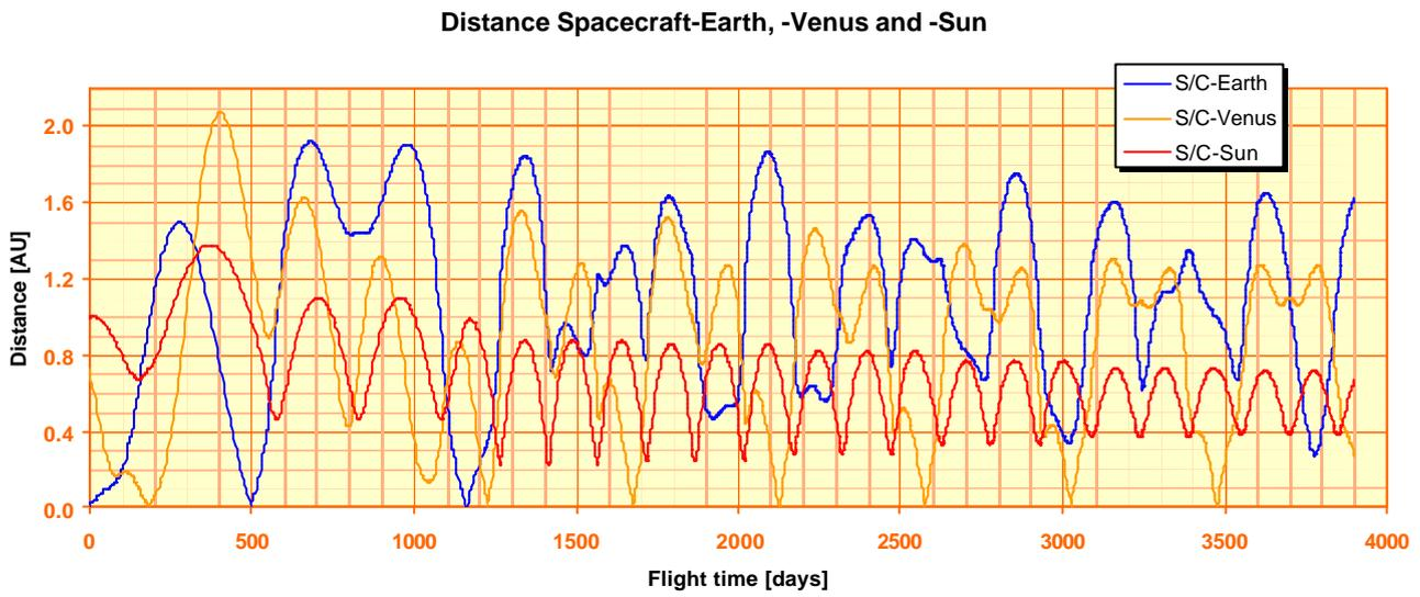
Figure 2-4. Ballistic transfer, 2013 launch: distance of the spacecraft from Earth, Venus and Sun function of flight day.
