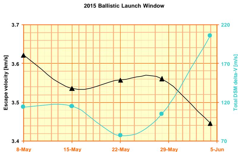
Figure 2-33. Variation in escape velocity and total DSM  $DV$  for optimum launches between May 8 and June 4, 2015.
