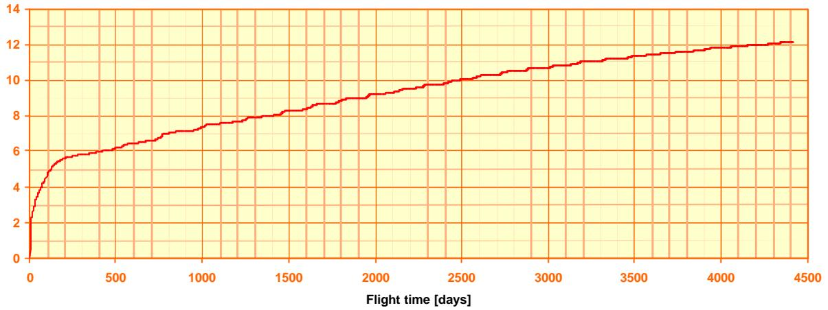
Figure 2-30. Ballistic transfer, 2017 launch: solar radiation integrated doses function of flight day.
