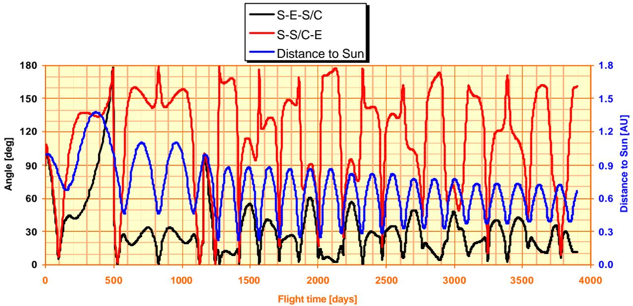
Figure 2-5. Ballistic transfer, 2013 launch: angle Sun-Spacecraft-Earth and Sun-Earth-Spacecraft and distance to Sun centre [AU] function of flight day.
