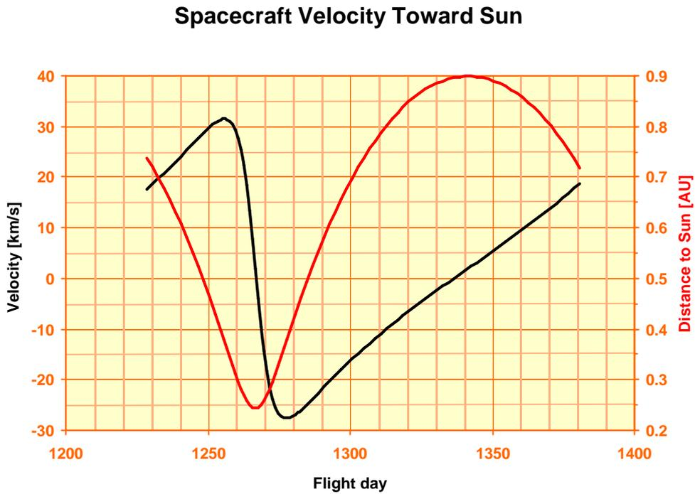
Figure 2-9. Ballistic transfer, 2013 launch: velocity toward the Sun [km/s] and distance to Sun centre during first revolution after Venus GAM 2.
