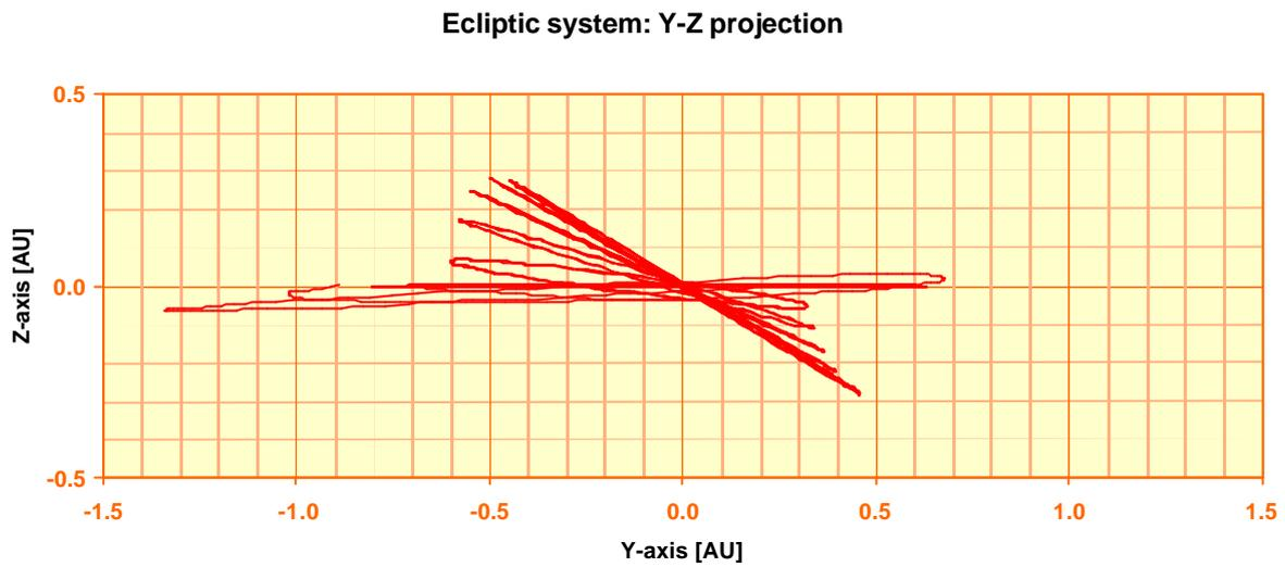
Figure 2-14. Ballistic transfer, 2015 launch: projection of the trajectory on the ecliptic system (y, z)-plane.
