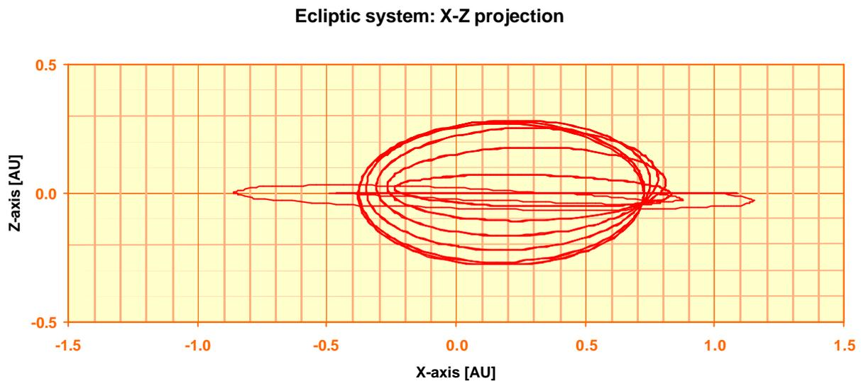
Figure 2-15. Ballistic transfer, 2015 launch: projection of the trajectory on the ecliptic system (x, z)-plane.
