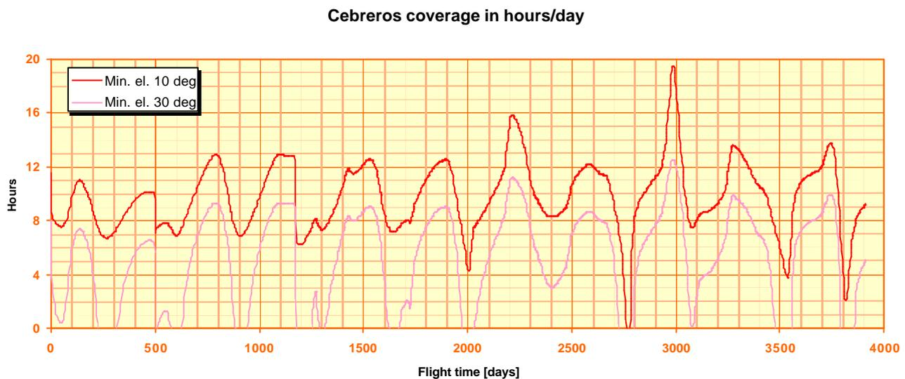
Figure 2-22. Ballistic transfer, 2015 launch: coverage in hours/day from Cebreros function of flight day.
