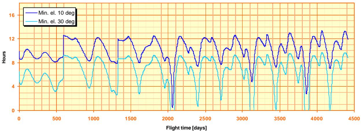
Figure 2-31. Ballistic transfer, 2017 launch: coverage in hours/day from New Norcia function of flight day.
