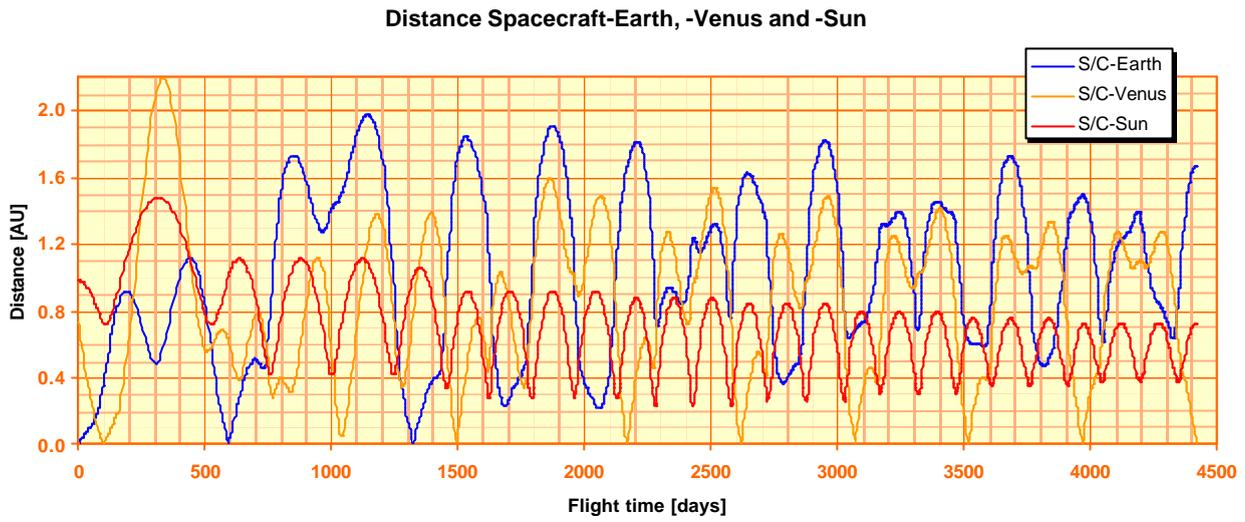
Figure 2-26. Ballistic transfer, 2017 launch: distance of the spacecraft from Earth, Venus and Sun function of flight day.
