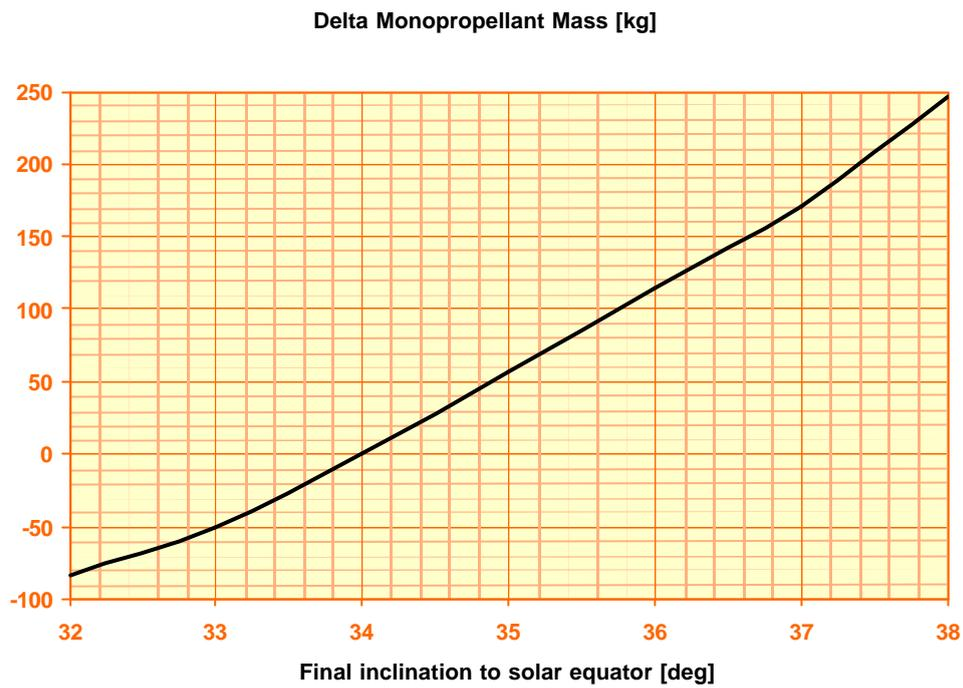
Figure 3-3.  $\Delta$ -monopropellant mass in terms of the reachable final inclination relative to the solar equator for a CP mission.
