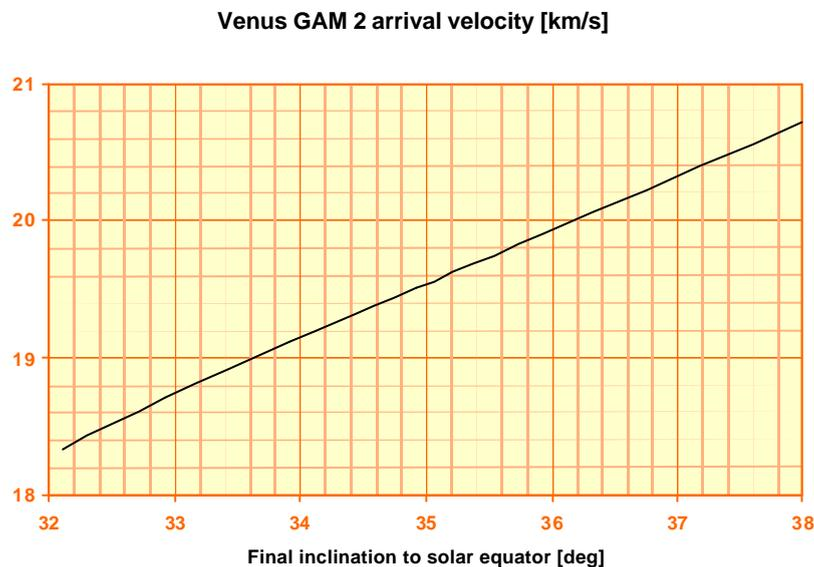
Figure 3-2. Arrival hyperbolic velocity at Venus GAM 2 in terms of reachable final inclination with respect to solar equator for the 2013 ballistic mission.
