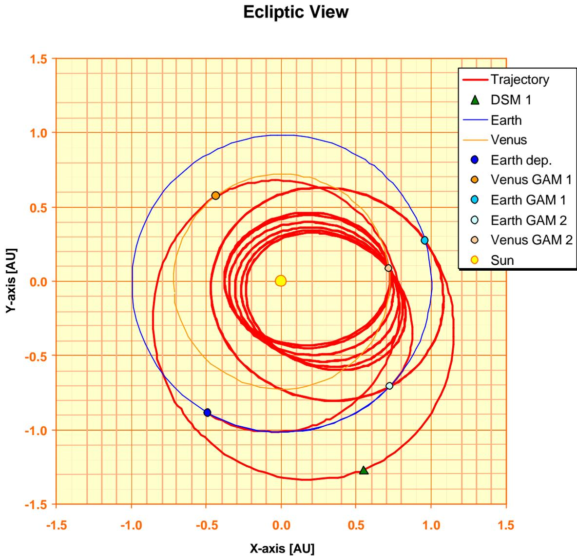
Figure 2-13. Ballistic transfer, 2015 launch: ecliptic view of the trajectory, GAMs until Venus GAM 2 and DSMs.
