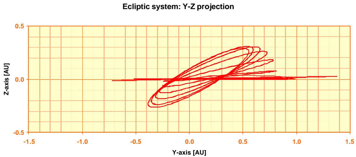
Figure 2-2. Ballistic transfer, 2013 launch: projection of the trajectory on the ecliptic system (y, z)-plane.
