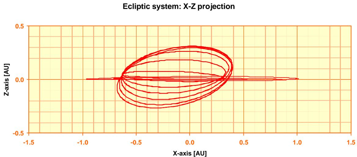
Figure 2-3. Ballistic transfer, 2013 launch: projection of the trajectory on the ecliptic system (x, z)-plane.
