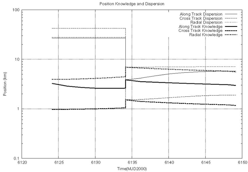
Figure 4-4. Evolution of the  $1\sigma$  position knowledge (thick lines) and dispersion (thin lines) mapped to the pericentre (GAM V3).
