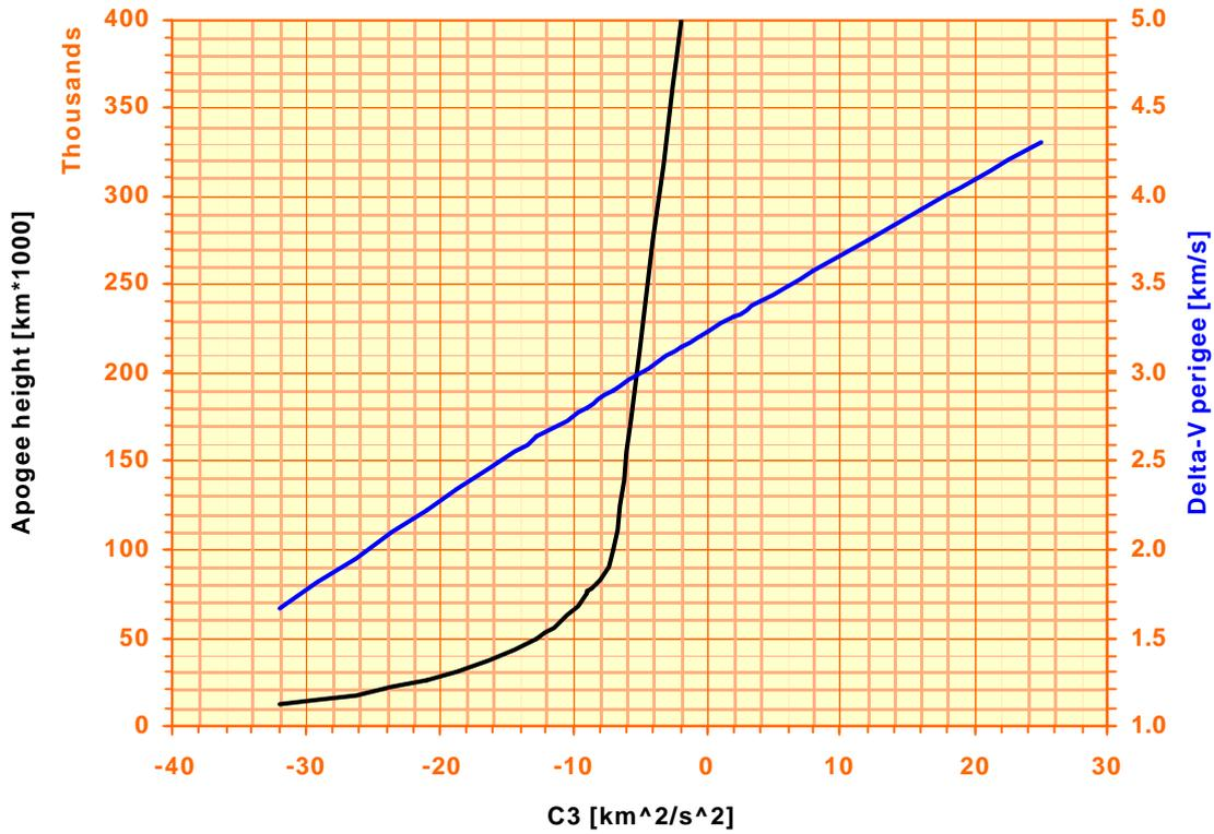
Figure 5-2. Correspondence between  $C_3$  and apogee height (black curve) and perigee injection  $DV$  (blue curve).
