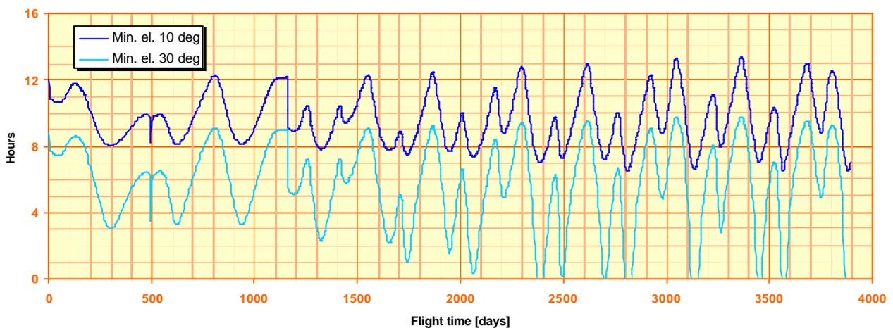
Figure 2-11. Ballistic transfer, 2013 launch: coverage in hours/day from New Norcia function of flight day.
