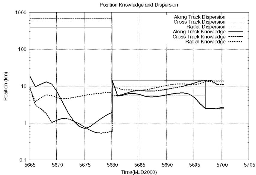
Figure 4-1. Evolution of the  $1\sigma$  position knowledge (thick lines) and dispersion (thin lines) mapped to the pericentre (GAM V2).
