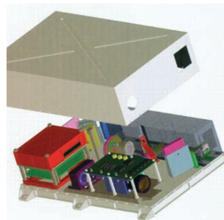
Fig. 1. Layout of the UV and IR channels. The IR AOTF spectrometer is at front left; the UV spectrometer is at the back. The common optical axis points to the right (+Z spacecraft axis).
