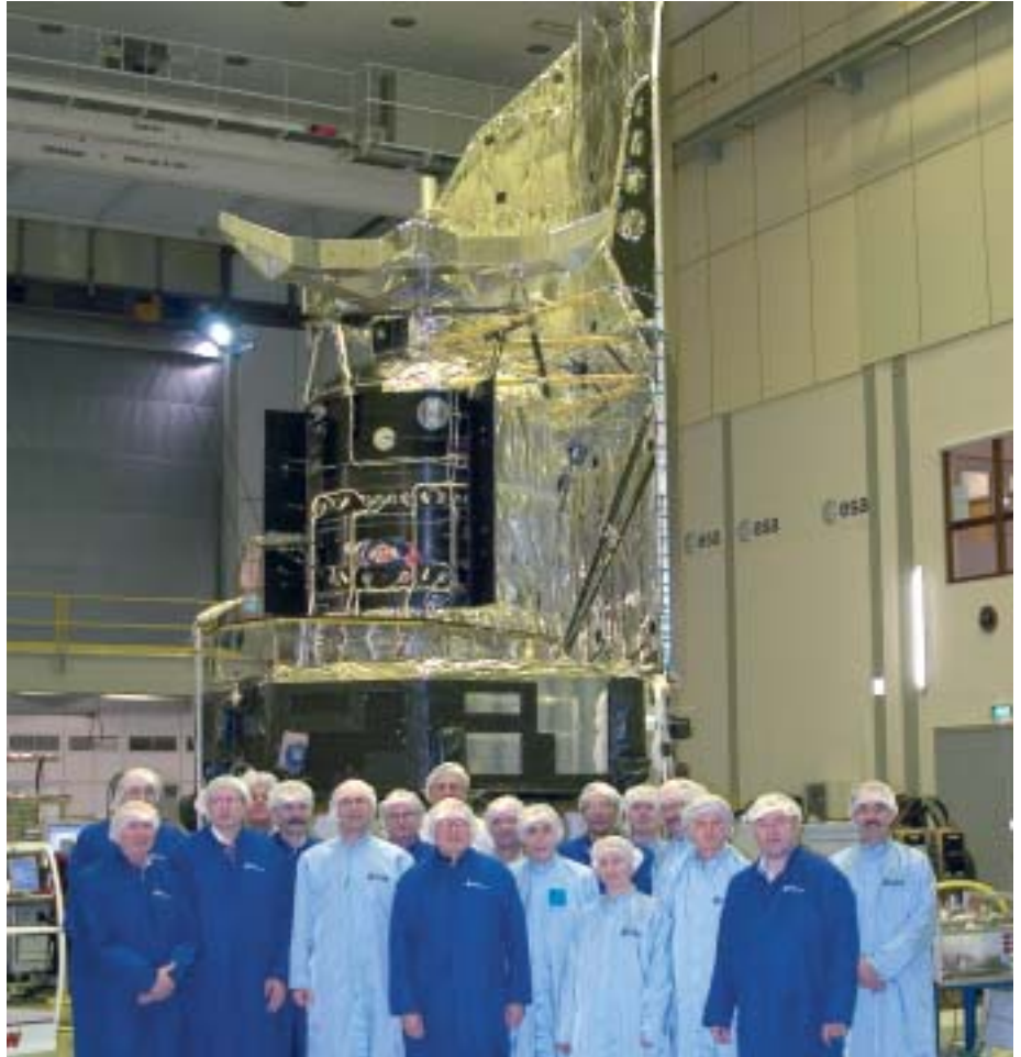
Figure 4.1.1. Herschel during the mechanical qualification campaign in the ESTEC Test Centre. The cryostat (with the black radiator in the centre), six of the eight side panels plus the top and bottom panels of the service module, the thermal shield and the upper half of the sunshade are flight hardware. The photograph was taken on 1 February 2006 during a Herschel Science Team meeting.
