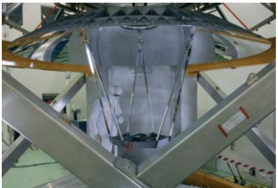
Figure 4.1.2. The Herschel telescope, shown during warm alignment activities at Astrium in Toulouse (F) in summer 2005. (EADS Astrium)
