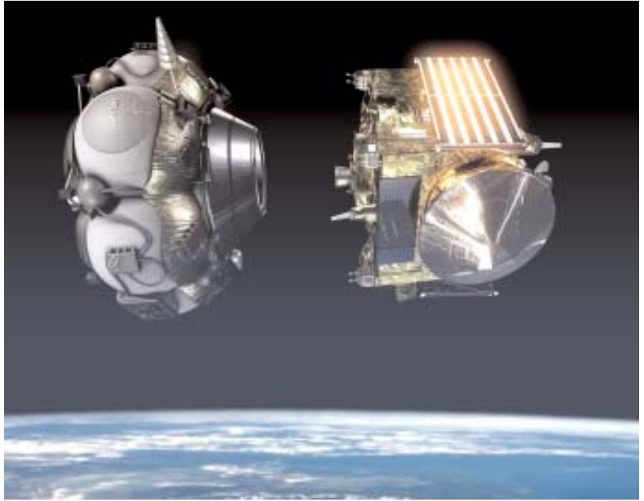
Figure 2.12.2. Venus Express separates from its upper stage after the second burn of the Fregat engine that has injected the combination into a heliocentric orbit towards Venus. The solar panels were deployed a few minutes later.
