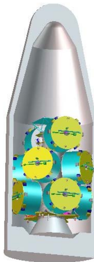
Figure 19: Cross-Scale composite within Soyuz-ST fairing.
