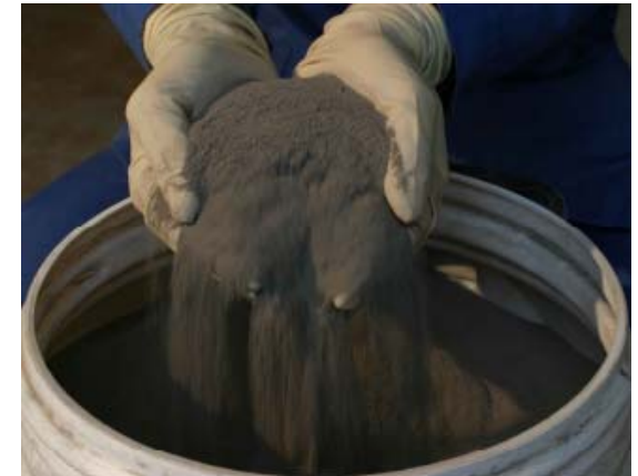
> From SiC "dust" to a cryogenic fully formed 3.5 m diameter Telescope !
