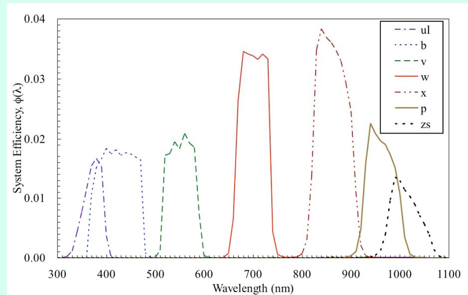
The system efficiency of AMICA seven band filter.
