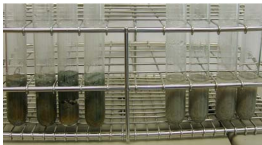
Figure 2. Microenvironments showing possible indications of Fe 0 oxidized to the Fe 3+ state. All tubes are identical with the exception of 1 gram of Fe 0 added to the four tubes on the left.
