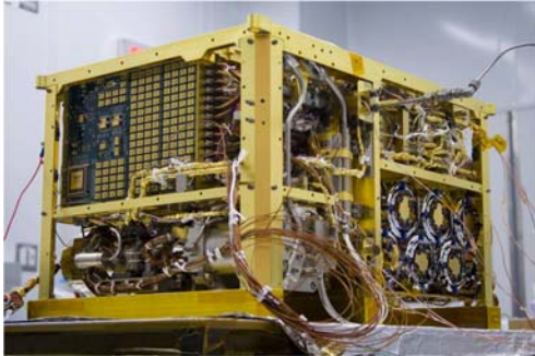
Figure 1: TLS (cylindrical spectrometer across the lower left) is mounted in the SAM structure).
