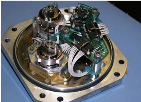
Figure 2: The two laser sources with triple-lens collimators are mounted to the 4-inch square laser plate ready for insertion into the spectrometer.
