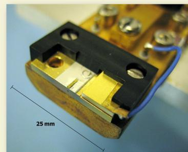
7.7  $\mu\text{m}$  QCL mounted on a substrate and installed in a custom made laser head
