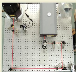
Setup of the optical bench during testing of the 7.7  $\mu\text{m}$  QCL at the Rutherford Appleton Laboratory
