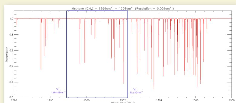
High resolution (0.001 cm<sup>-1</sup>) simulated CH<sub>4</sub> spectrum from 1296 - 1308 cm<sup>-1</sup> with the 7.7  $\mu\text{m}$  QCL tuning range shown in blue
