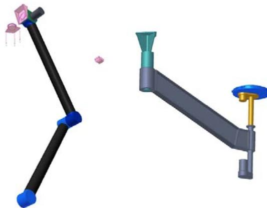
Figure 12: Sampling Arm and Closing Arm
