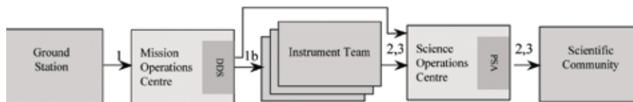
Fig. 1. The data flow from the ground station in New Norcia, Australia, to the scientific community. The numbers above the arrows indicate the data processing levels. Iterations that might occur in the data flow are not indicated.
