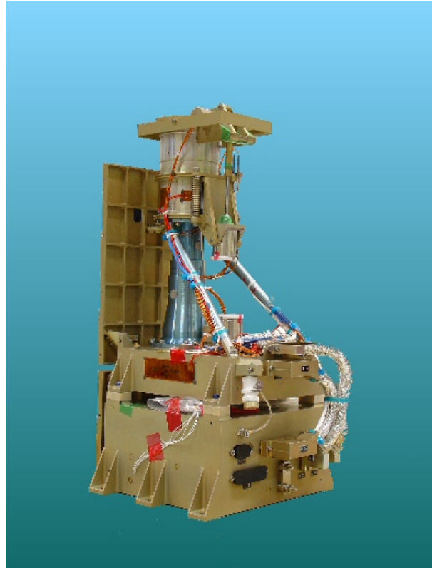
Figure 6-1. Framing camera for the DAWN mission as representative instrument, providing heritage for NAC (Credit: MPS, DLR)
