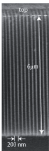
Figure 4.28. Scanning electron micrograph of a cleaved cross section through a 200 nm-period CAT grating.
