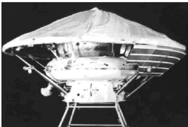
Figure 1. The Mars 3 lander (V.G. Perminov, the difficult road to Mars), the lander included complicated scooping mechanisms and symbolic objects including a Soviet pennant, the cleans spacecraft operated a few seconds on the surface while its sister spacecraft crashed without emitting telemetry. The cleansing procedures of the time did not involve baking.
