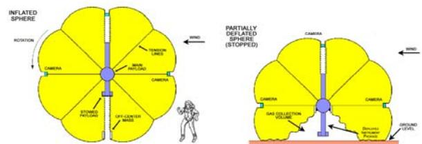
Figure 1. Inflatable Tumbleweed based upon airbag technology developed at JPL.
