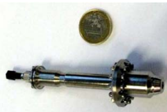
Figure 13: Nd-YAG Laser of LIBS prototype for ExoMars, Pasteur.
