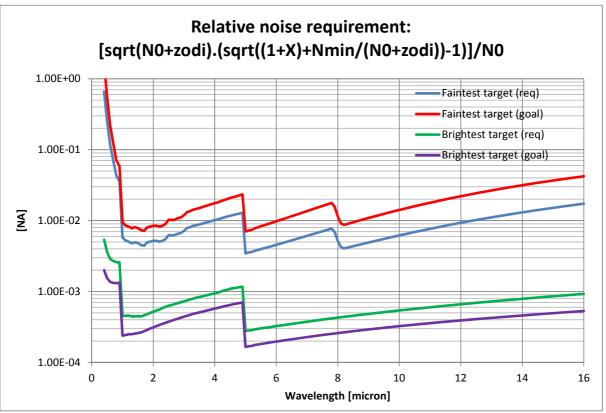
The system level noise (post-processing) is given in Figure 8 relatively to the stellar flux:
