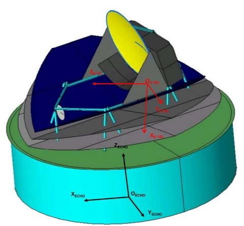
**Figure 9:Definition of the EChO reference frames**
