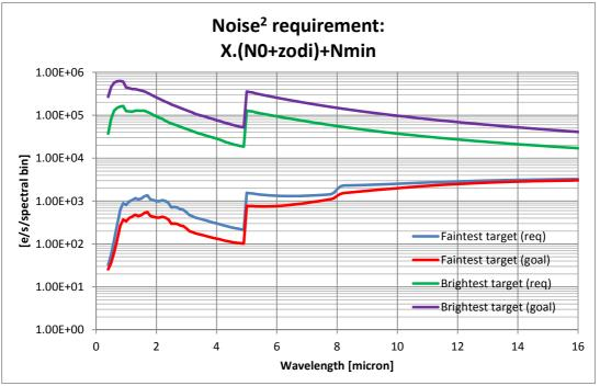
Figure 7: Square of noise requirement (to be summed in RSS with the noise floor)
