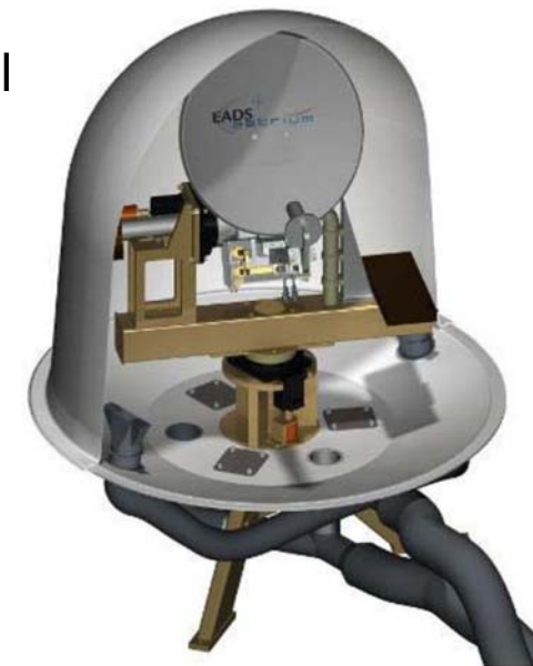
MWL ground terminal (2 - 3 m dish)
