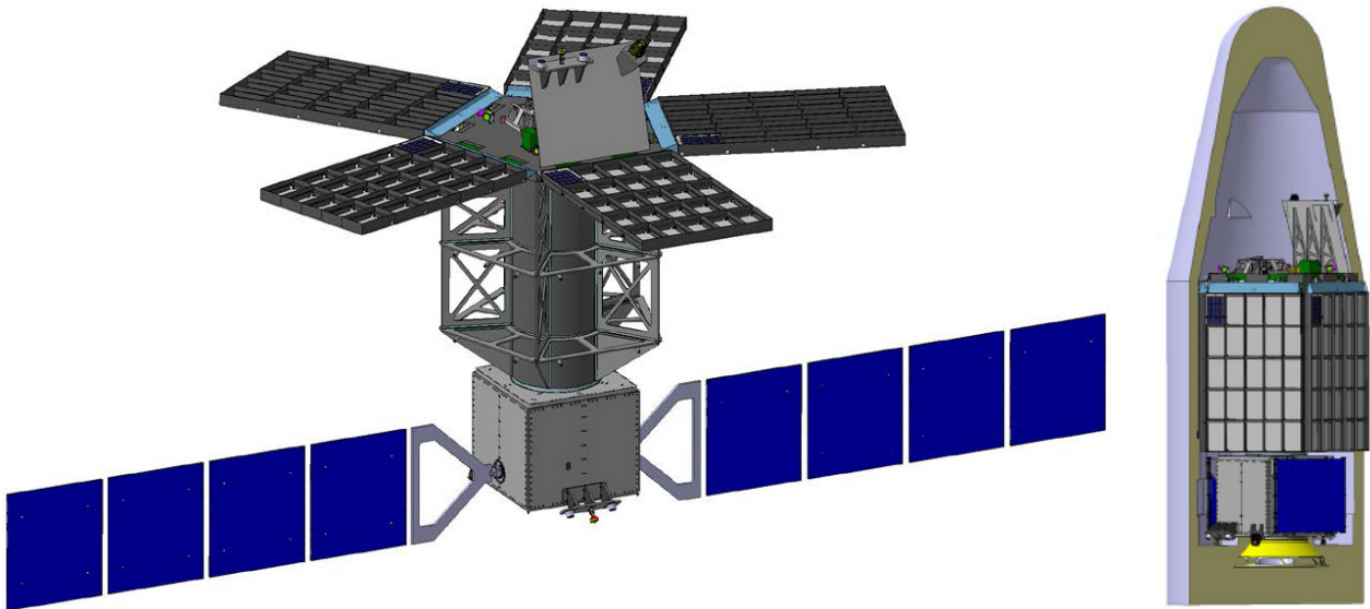
Figure 5-2 View of the LOFT SC concept [A] in the deployed (left) and stowed (right) configuration. This design assumes 5 panels with each 25 modules and one PBEE per panel.
