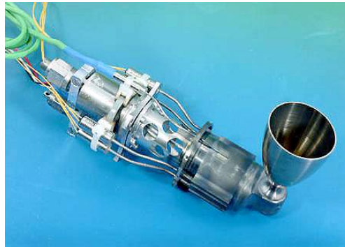
Figure 13-9: Model CHT-20N thruster developed by EADS (DE)
