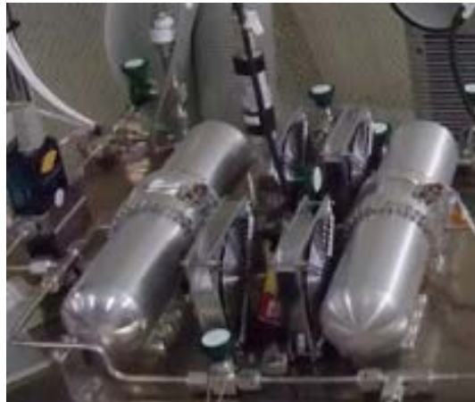
Figure 10-1: JAXA Joule-Thomson cooler
