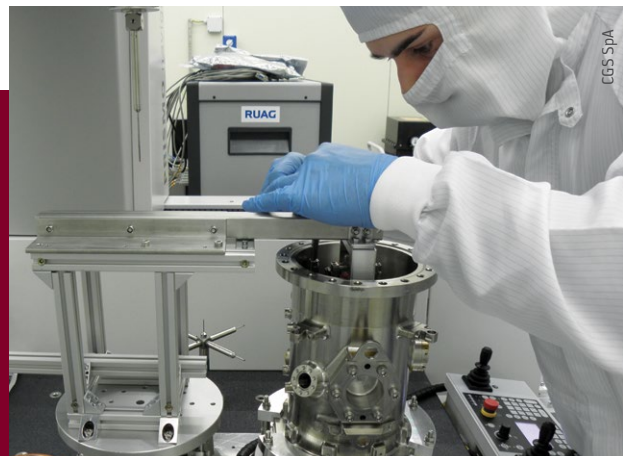
Checking alignment on one of the inertial sensor heads for the LISA Technology Package
