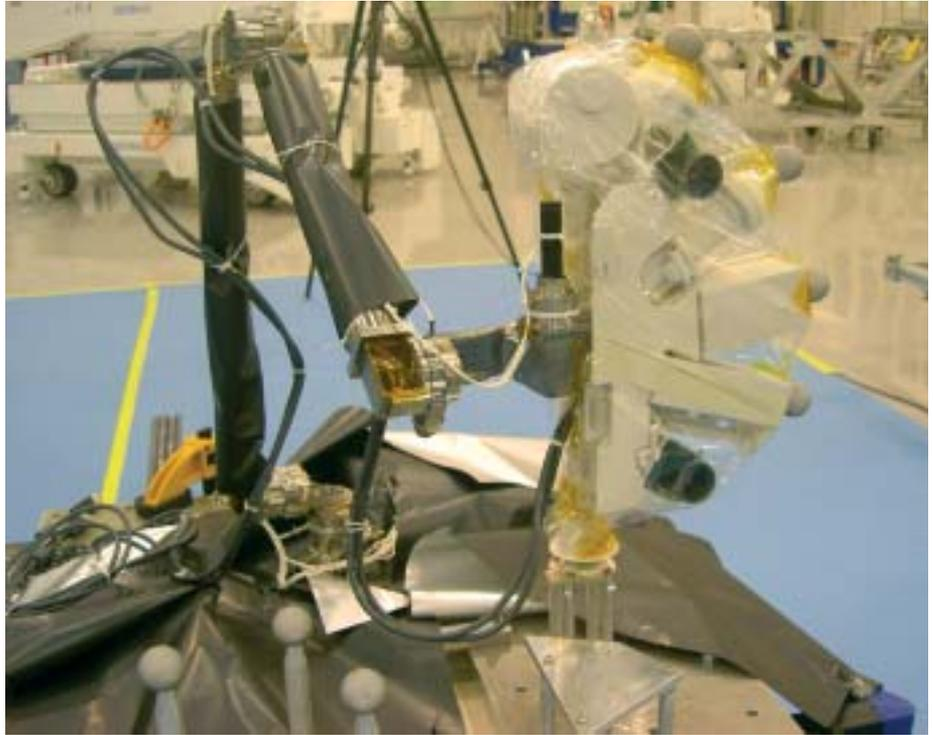
ARM operations that are deemed to be 'safe points'. These are configurations that can be returned to at any time without risk of collision and from which a series of pre-set manoeuvres can be initiated.
