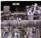
The Gaia torus during installation of one large mirror http://sci.esa.int/gaia/58208
