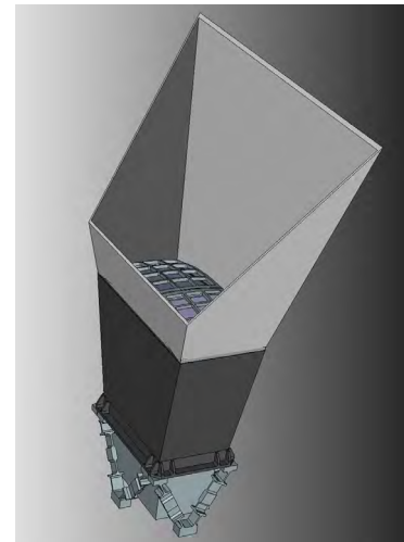
Fig. 10: CAD drawing of the SMILE SXI as viewed from the top. Clearly visible are the micropore optic arrays, protected from stray light by the baffle. X-rays are focussed onto CCDs located at the bottom of the (black) optical bench.
