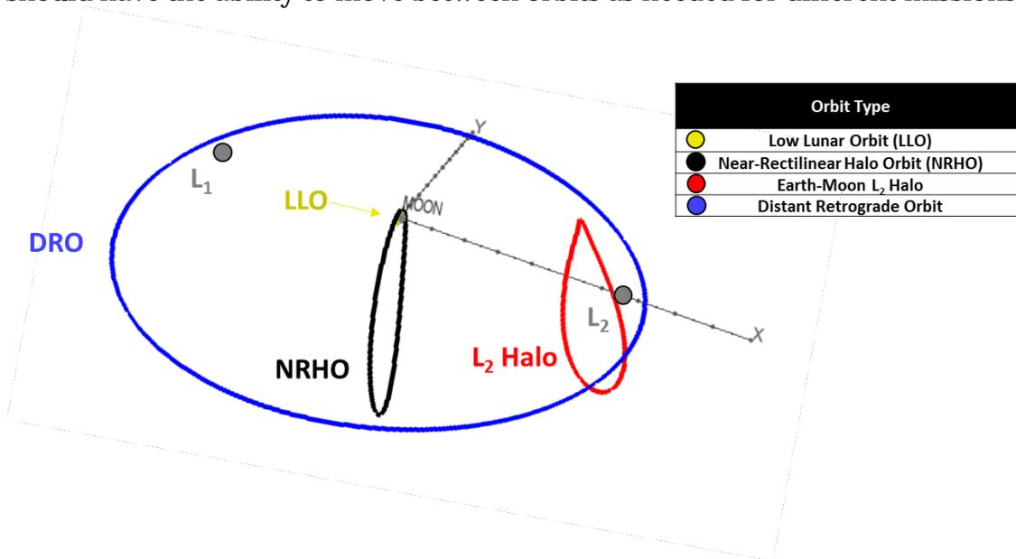
Figure 1 Orbit types reviewed for the Deep Space Gateway. Of those reviewed Near Rectilinear Halo Orbits and Earth-Moon L<sub>2</sub> Halo orbits were found to be technically favourable.
