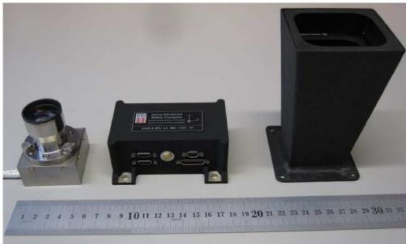
Figure 14-15: DTU Masc star tracker (left: Camera Head Unit, middle: DPU, right: baffle)
