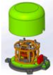
Figure 4-9: Probe B2 FGM sensor schematic
