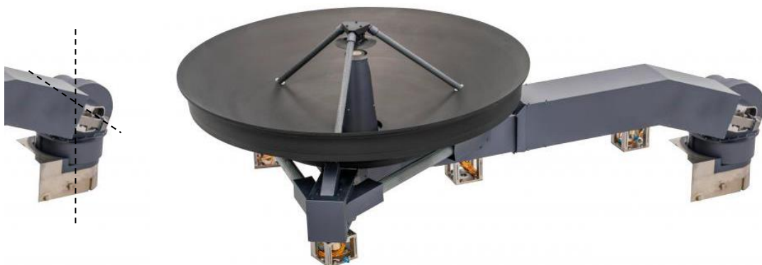
Figure 12-4: Picture of the baseline design Antenna pointing Mechanism in the Solar Orbiter configuration HGAMA
