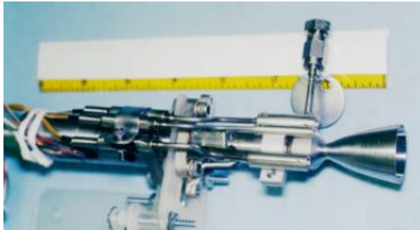
Figure 10-3: 5N thruster MONARC-5. Photo courtesy of MOOG Isp RD[21]
