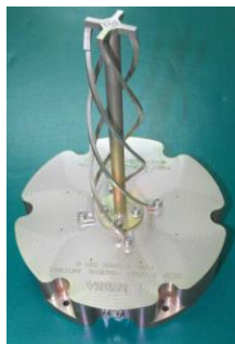
Figure 16-23 – S-band ISL toroidal antenna (Sener Aerospacial)
