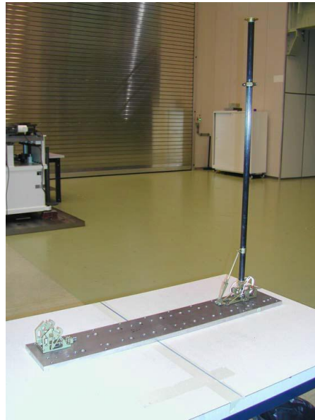
Figure 4-2: The VeX magnetometer boom under test at ESTEC's test facility
