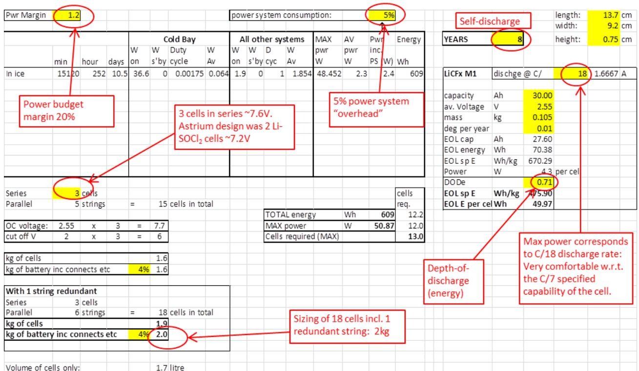
Figure 14-2: Annotated battery sizing spreadsheet (Penetrator)
