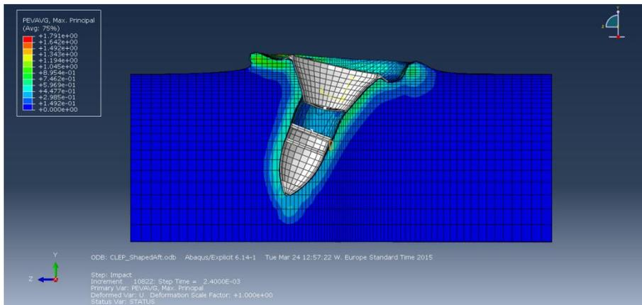
**Figure 10-4: Oblique spin stabilised impact with conical after body after 2.4ms**
