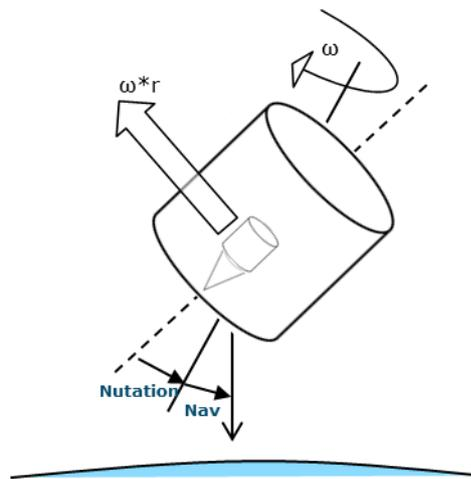
**Figure 13-7: Separation of penetrator during free-fall**
