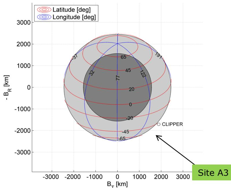
**Figure 5-8: Arrival conditions at Europa as seen in the B-plane. The dark grey area indicates the radius of Europa, the light grey area all the points that will lead to an impact when targeted. The corresponding level lines of landing latitude and longitude are also shown**
