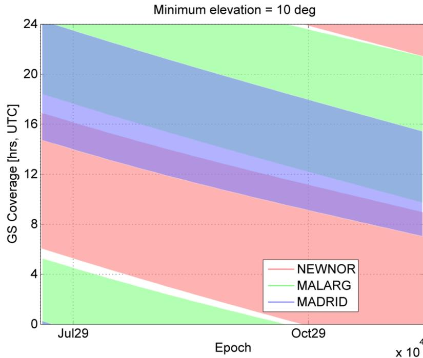
**Figure 5-6: Ground station coverage for the baseline transfer trajectory**
