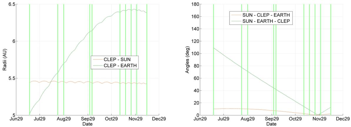
**Figure 5-4: Evolution of the distances to the Sun and the Earth as well as the relevant angles for the baseline transfer trajectory from 13E7 to a minimum V-infinity orbit**
