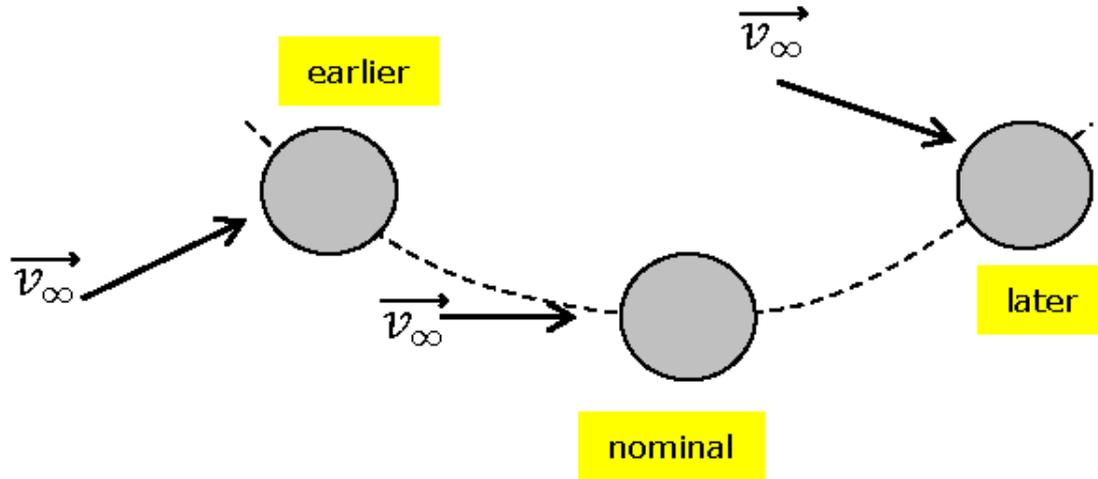
**Figure 5-19: Effect on V-infinity direction and magnitude for earlier/later arrival.
