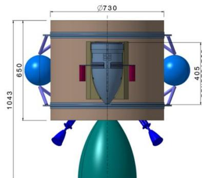
**Figure 17-1: PDS Configuration for the CLIPPER study (Courtesy of Airbus DS)**
