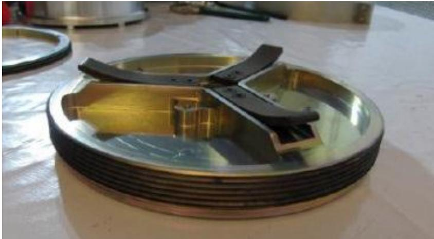
**Figure 17-6: Example of Torlon Springs used in the design (Courtesy of Airbus DS)**
