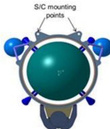
**Figure 11-1: PDS to Clipper mounting points (Courtesy of Airbus DS)**
