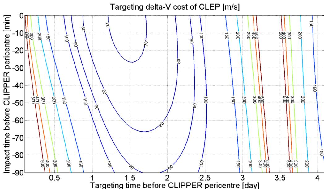
**Figure 5-13 Targeting  $\Delta V$  magnitude with different targeting and arrival times**
