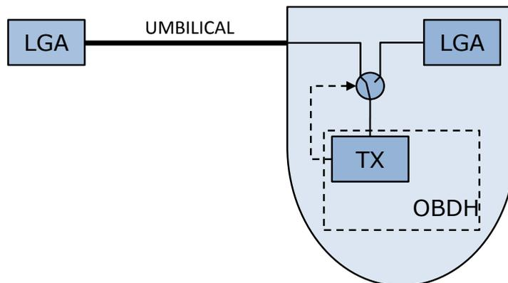
**Figure 16-4: Penetrator Communication S/S**
