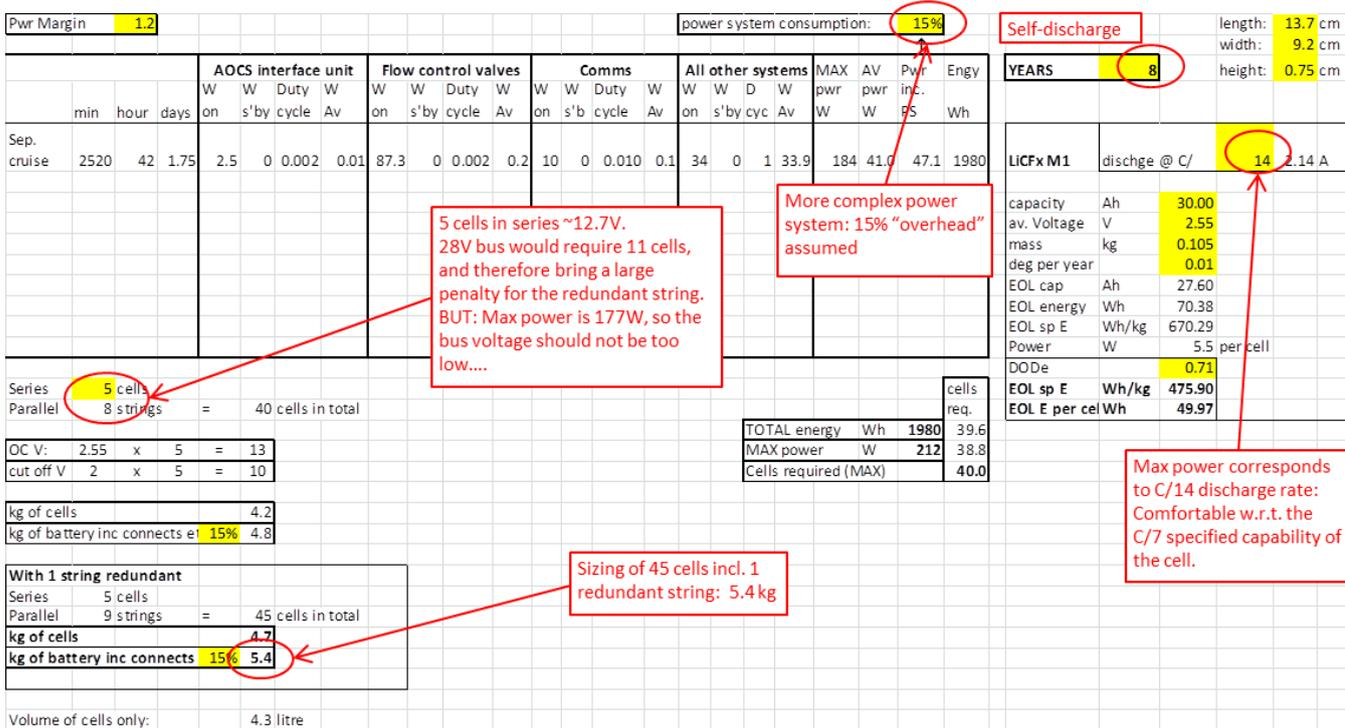
Figure 14-3: Annotated battery sizing spreadsheet (PDS)
