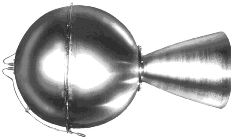
**Figure 12-4: STAR 24 Solid Propellant Rocket Motor**
