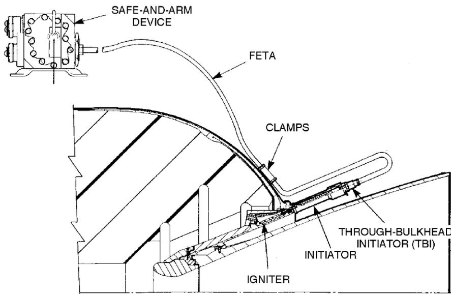
**Figure 12-6: Typical STAR solid propellant rocket motor ignition train**
