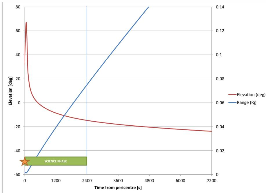
**Figure 16-1: Visibility vs data generation during second fly-by**
