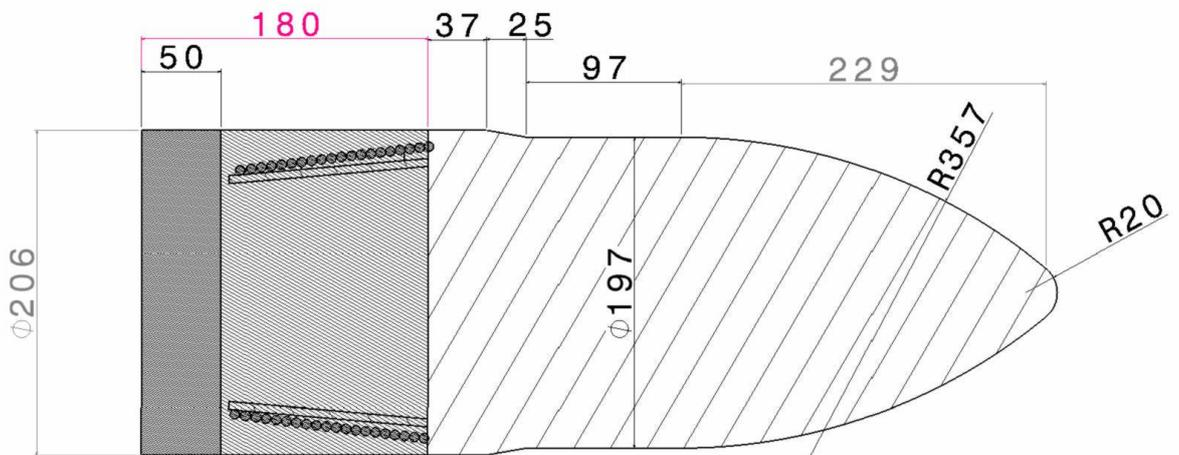
**Figure 9-7: Penetrator overall dimension**
