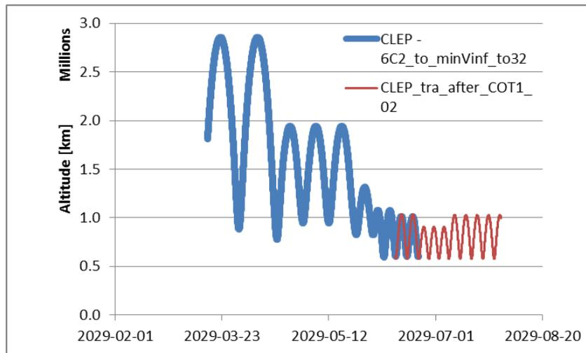
Figure 8-1: CLEP altitude as function of time
