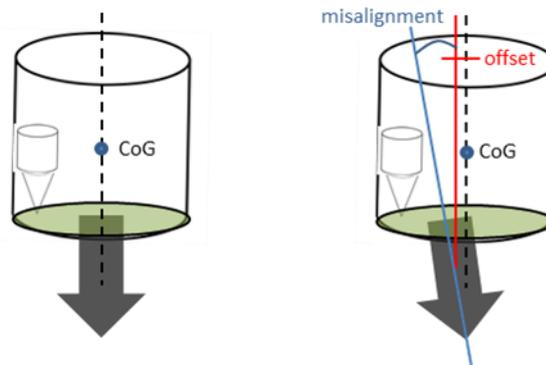
**Figure 13-4: Nominal and actual SRM thrust direction**
