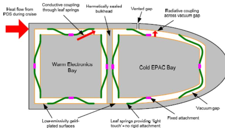
Figure 5-17 Proposed Penetrator thermal concept
