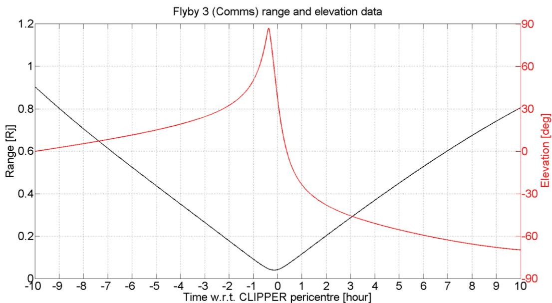
**Figure 5-12 Range (black) and elevation (red) plots for the 2nd fly-by**
