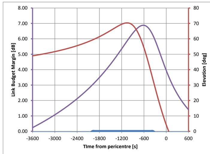
**Figure 6-11: CLIPPER visibility Fly-by 3 - Link budget**
