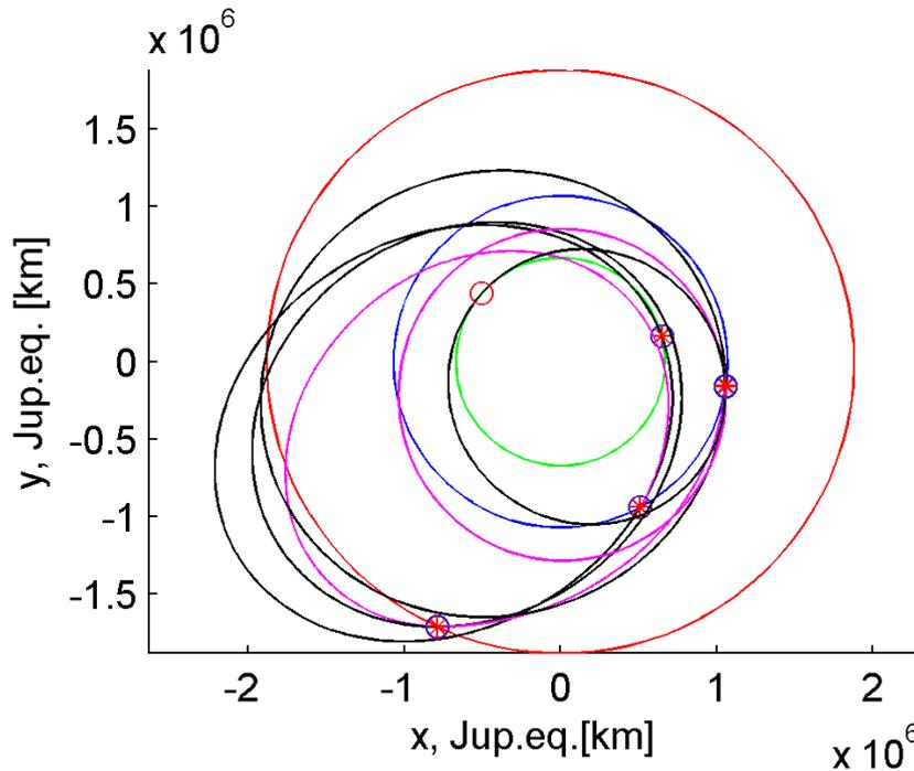
**Figure 5-1: Transfer trajectory from after COT-1 to minimum V-infinity orbit.**
