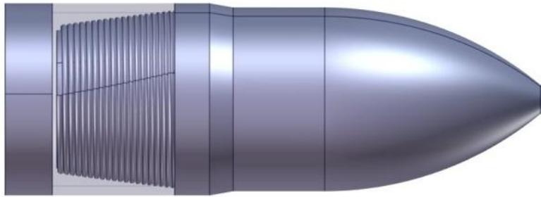
**Figure 9-5: Penetrator design including the aftbody**
