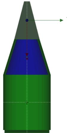
**Figure 8-4: CLEP penetrator model for ray tracing**
