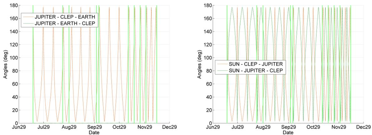
**Figure 5-5: Evolution of Jupiter-CLEP-Earth and Sun-CLEP-Jupiter geometry for the baseline transfer to a minimum V-infinity orbit**
