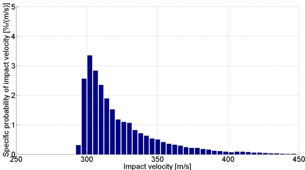
**Figure 5-14 Total impact velocity dispersion with targeting measurement**
