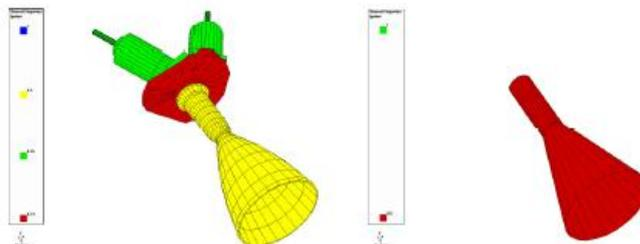
**Figure 17-3: Detailed and Reduced Thermal Model of Lunar Lander small Thruster (Courtesy ADS)**
