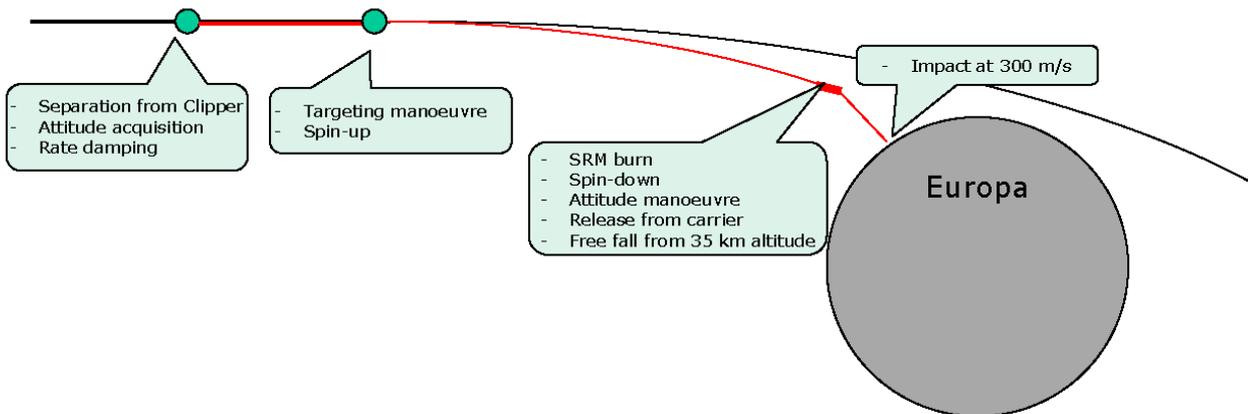
**Figure 5-9: Time line overview of the CLEP final approach (schematic)**
