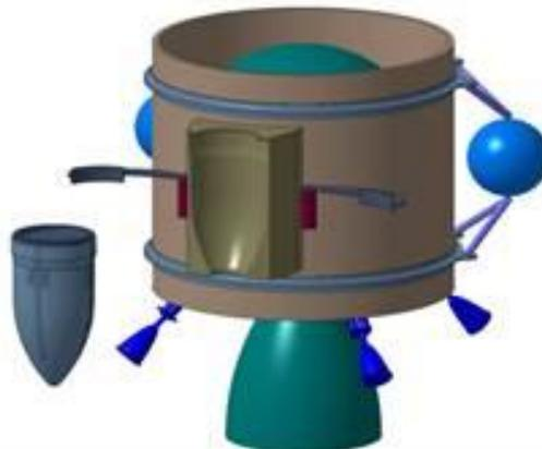
**Figure 11-3: Separation Mechanism (Courtesy of Airbus DS)**
