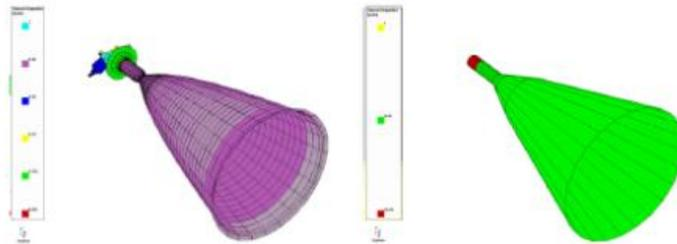
**Figure 17-4: Detailed and Reduced Thermal Model of Lunar Lander Main Engine (Courtesy ADS)**
