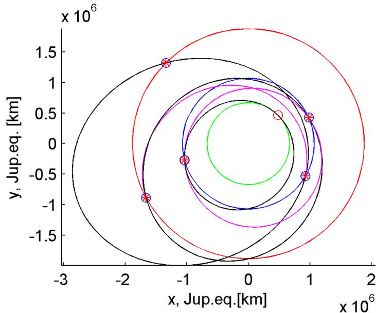
**Figure 5-17: Transfer trajectory from 6C2 to a minimum infinite velocity w.r.t. Europa (option).**
