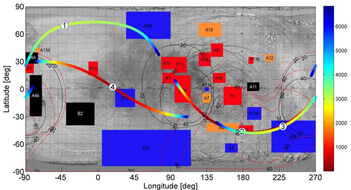
**Figure 5-10: Ground tracks on the surface of Europa of the baseline fly-by sequence. The number labels indicate the pericentre of the fly-by. Only parts of the fly-by  $\pm 1h$  to CLIPPER pericentre are plotted. The altitude is indicated by the colorbar. Black contour lines enclose regions in which CLIPPER's elevation is higher than  $30^\circ$  for the indicated number of minutes at the 2<sup>nd</sup> fly-by. Red contours show the same for the 3<sup>rd</sup> fly-by**
