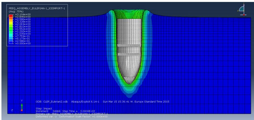
**Figure 10-1: Vertical impact penetration with ductile ice model**
