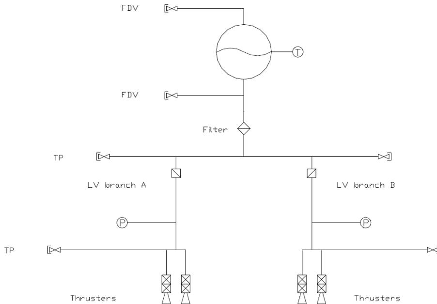
**Figure 12-1: Hydrazine baselined propulsion system architecture**
