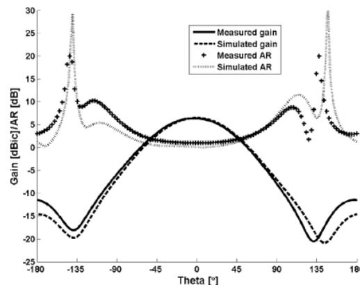
Fig. 13. Measured and simulated gain and axial ratio in *XZ*-plane at 1.605 GHz.
