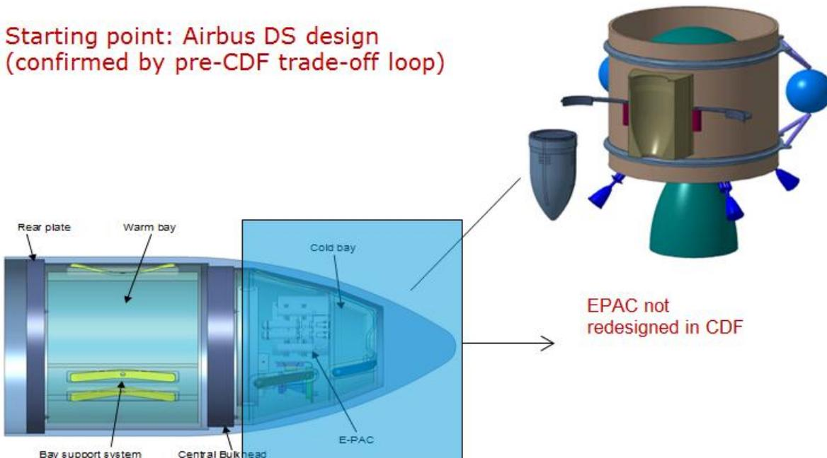
**Figure 6-1: Airbus PDS & Penetrator Design (Courtesy of Airbus DS)**
