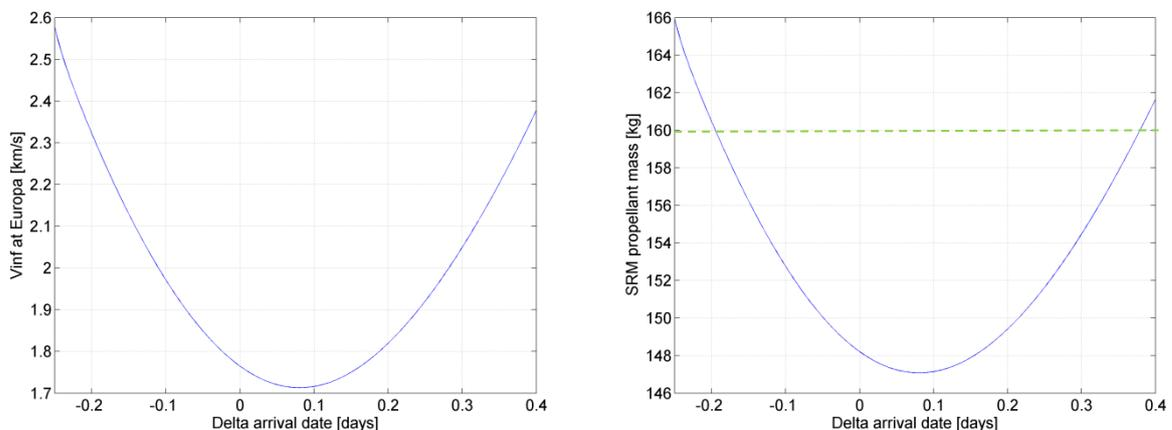
**Figure 5-18: Arrival infinite velocity at Europa and corresponding SRM propellant mass as a function of the arrival date**
