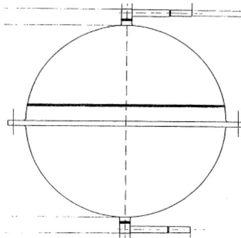
**Figure 12-3: PEPT 230: Selected propellant tank**
