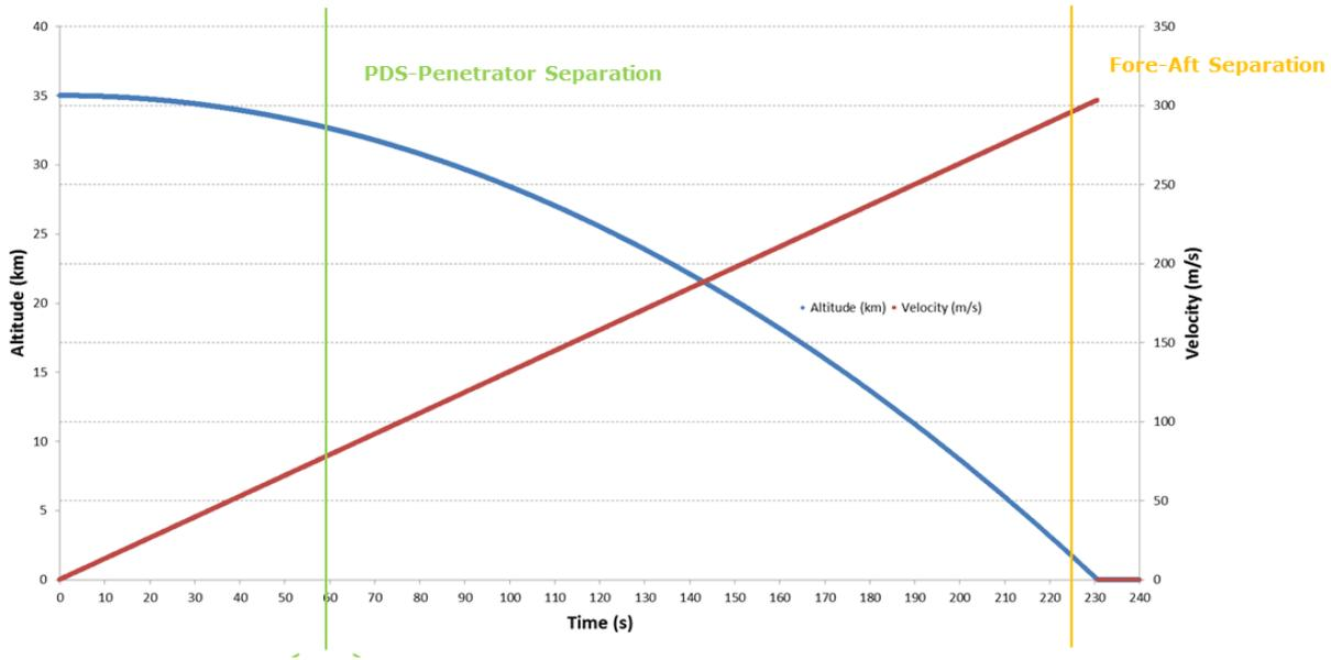
**Figure 6-8: PDS & Penetrator Free Fall: separation events planning**
