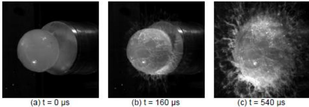
**Figure 10-2: Hail Impact test results RD[12]**
