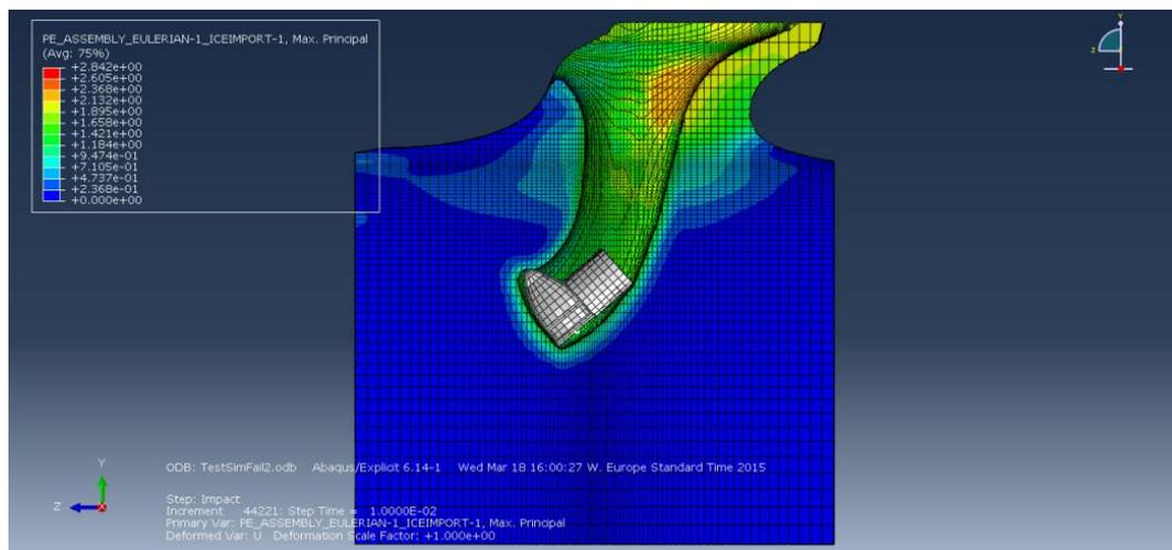
**Figure 10-3: Oblique impact with detachable after body and brittle ice model**
