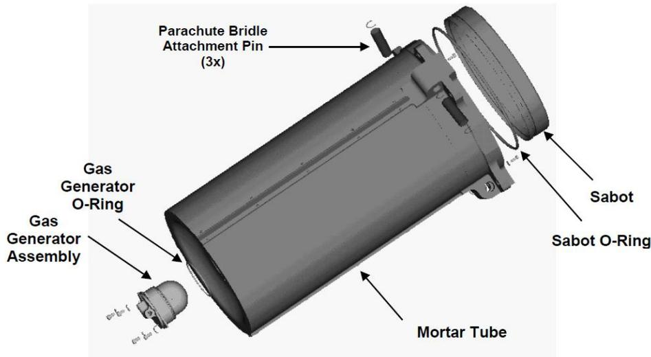
**Figure 11-5: Typical configuration of a Parachute deployment system**
