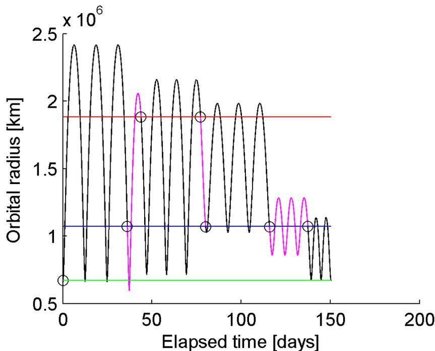
**Figure 5-2: Evolution of the orbital radius of the baseline transfer trajectory. Europa, Ganymede and Calisto orbital radii are drawn as green, blue and red lines. Fly-bys are indicated as circles**
