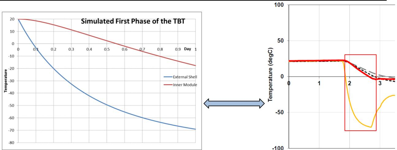
**Figure 17-8: Left – Results of the simplified thermal Model, Right – Excerpt of the Thermal Test Report**
