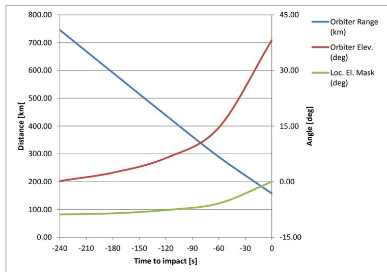
**Figure 16-3: Orbiter visibility from PDS during last phase of descent**
