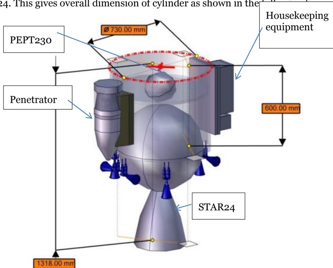
**Figure 9-2: Penetrator on PDS**
