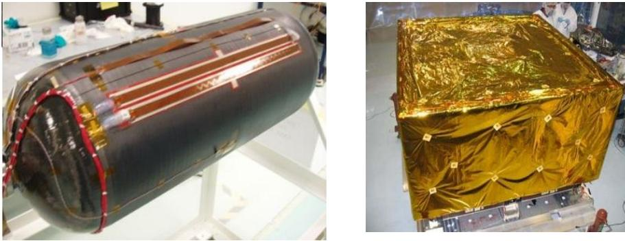
**Figure 17-2: Examples of items used for the TCS of the PDS – Left Kapton Heaters, Right MLI**
