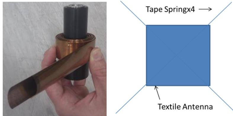
Figure 11-7: Tape spring(left) Textile antenna deployed (right)
