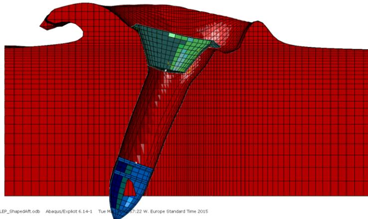
**Figure 6-2: Preliminary simulations. Penetrator with conical aft body**
