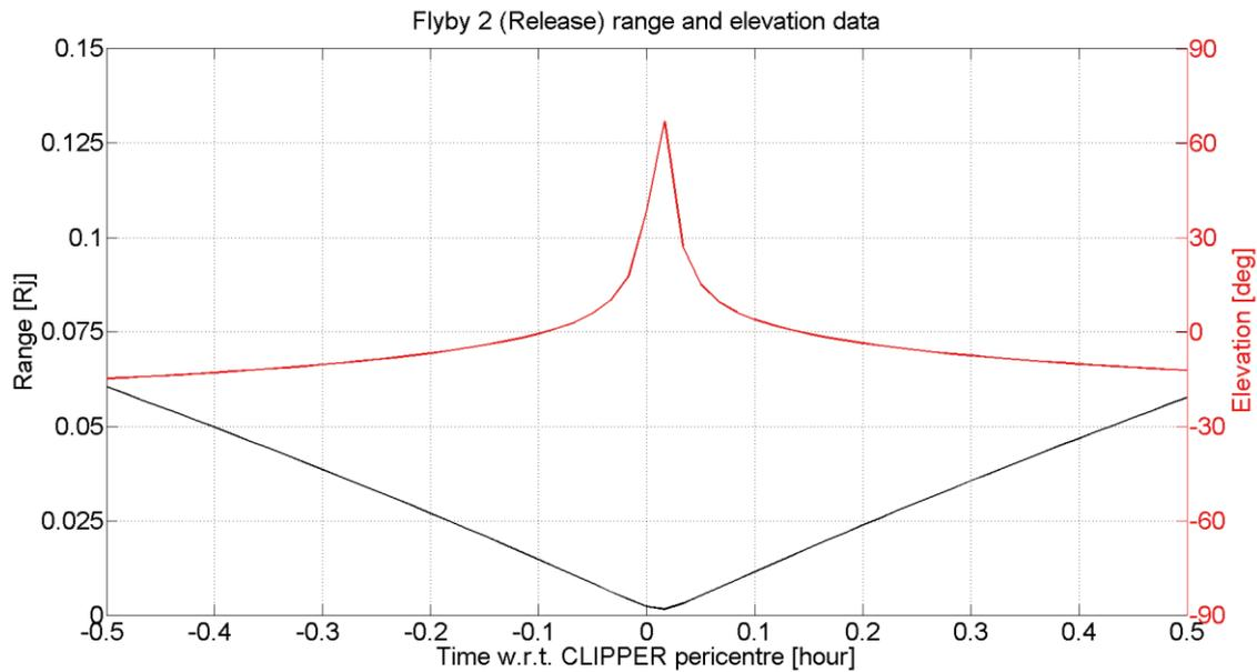
**Figure 5-11 Range (black) and elevation (red) plots for the 1st fly-by**
