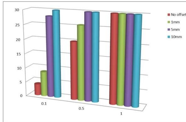
**Figure 13-5: Nutation angle wrt misalignment and offset at 50 rpm**
