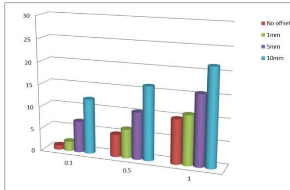
**Figure 13-6: Nutation angle wrt misalignment and offset at 100 rpm**
