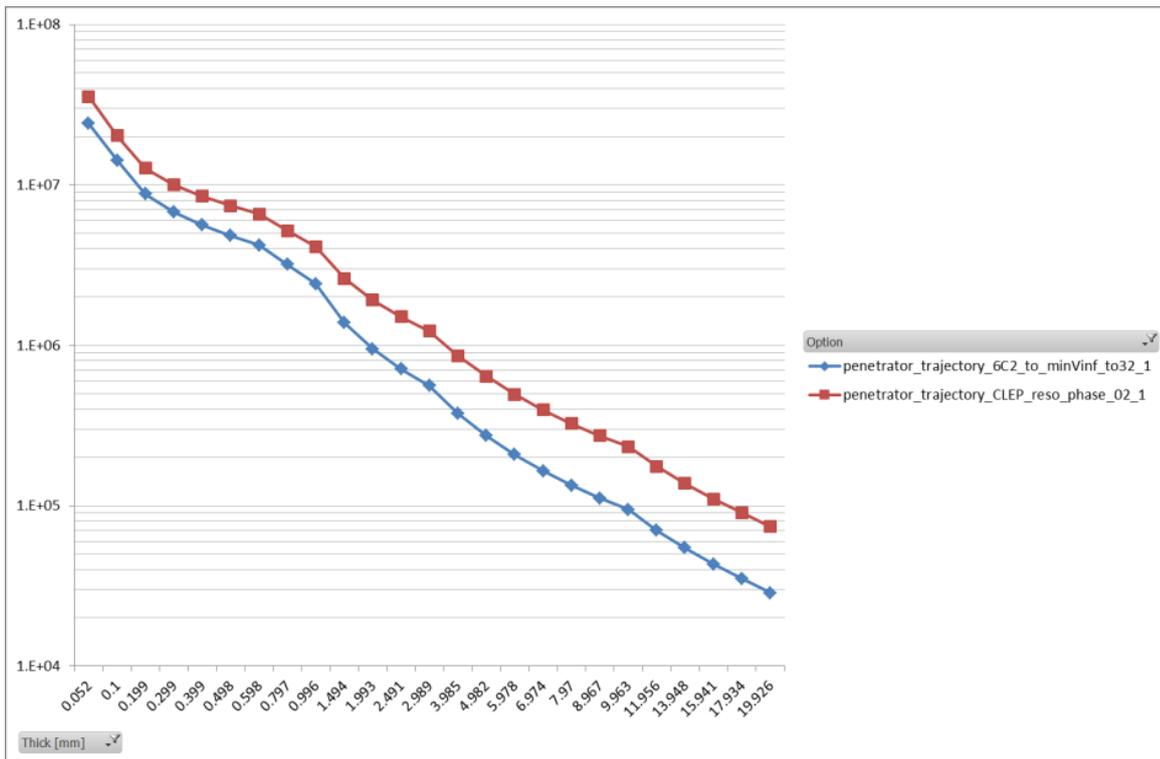
Figure 8-2: CLEP dose as function of shielding thickness
