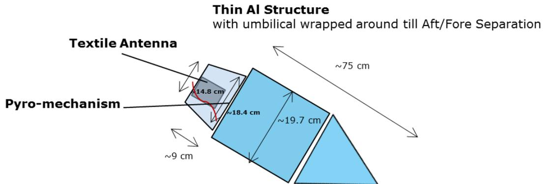
**Figure 6-3: Penetrator Baseline: Fore and Aft Bodies
