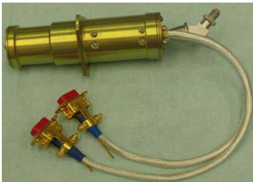
Figure 6-23: Cold thruster selected used on Gaia
