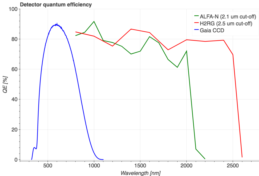
Figure 5-24: Comparison between different, measured detector quantum efficiencies: in blue the Gaia CCDs to show the enlargement of the considered wavelength range, in red the baseline H2RG US detector with a cut-off at 2.5 \mu\text{m} , and in green the ALFA-N detector developed by the CEA Leti in France in the context of an ESA technology development activity. Note that below 800 nm, an average QE of 70% or more can be obtained for the two MCT devices (by removing the substrate on which the MCT photosensitive layer is grown)
