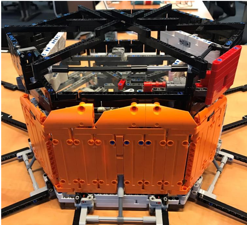
Figure 5-51: Focal plane assembly radiator (orange) with 6 m 2 size, FEE and DPU radiator (red) with 0.4 m 2 size
