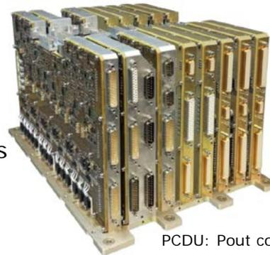
PCDU: Pout configurable with 3kW (max)
