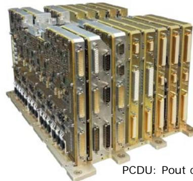
PCDU: Pout configurable with 3kW (max)
