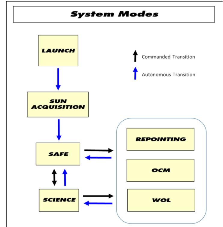
\* Additional Stand-by and Survival modes could be considered to, respectively, use RW instead of RCS (to minimize propellant use) or lower cryo-coolers duty cycle (to minimize power needs).
