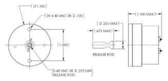
Note: Model 9100 Release Mechanism shown. Different configurations available with alternate release rods, mounting features, and connectors. Metric configurations are also available.
