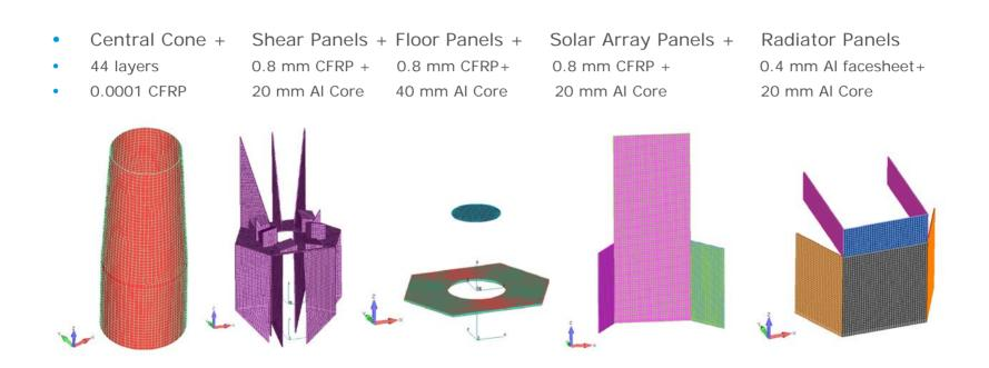
Structure Mass (Central Cone + Panels) = 540 Kg
