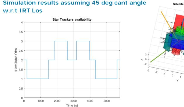
A reference orbit has been considered, with a fixed pointing towards North Pole at the edge of the FoR (theta = 40 deg)
