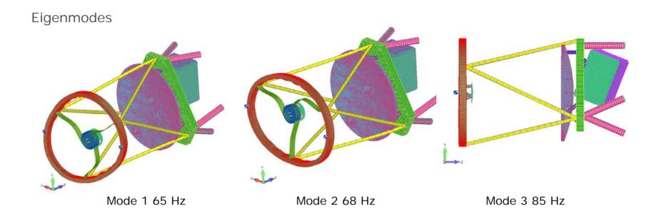
Eigenmodes 1 and 2 dominated by bending and torsional response of Upper Cage and M2 Spider. Eigenmode 3 dominated by rocking modes of spectrometer. Telescope Option 3 compliant with design mass and eigenfrequency requirements.
