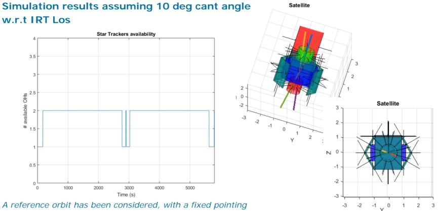
A reference orbit has been considered, with a fixed pointing towards North Pole at the edge of the FoR (theta = 40 deg)
