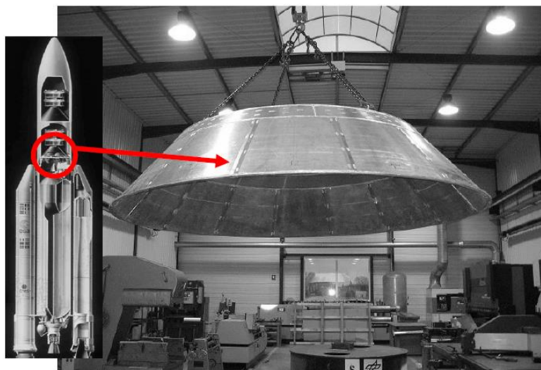
Figure 8-21: Payload adapter cone after assembly, from RD[13]
