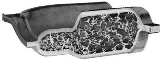
Figure 8-19: Bicycle crank arm, forged AFS parts and section (top image), tomogram of interior (bottom image), from RD[14]
