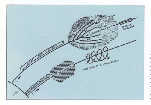
Schematic of suggested electrodynamic structure of near-Earth magnetosphere at auroral latitudes. An electric double layer accelerates downward (towards Earth) electron and upward ion beams and a consequent  $j_{\pm}$ . The return current is assumed to be carried by upwardly drifting cold electrons whose bulk energy feeds ion-cyclotron instabilities, which in turn accelerate H<sup>+</sup> and O<sup>+</sup> in the direction transverse to B (from Ashour-Abdalla & Okuda, 1982)
