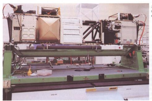
SPAS-01 during check-out at Kennedy Space Centre, showing the heat pipe flight verification experiment just left of centre.
