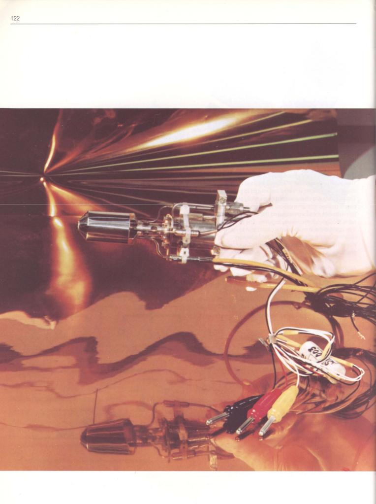
The 2-N thruster for use on board ISPM spacecraft. (Photo ERNO, Bremen).
