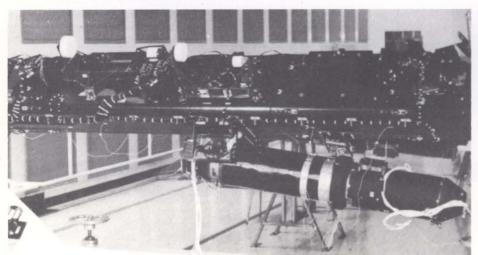
ISPM carbon fibre dish antenna (2 m).
